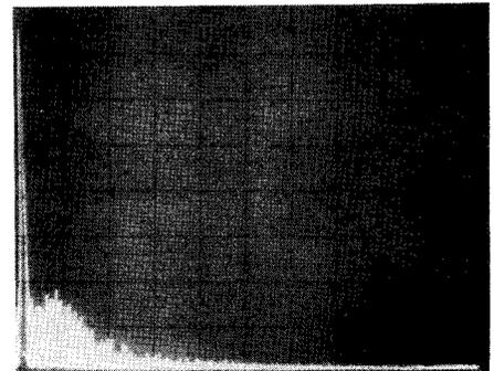
Fig. 2 — Spectral display of noise about the carrier frequency of the TS-830S. The carrier is at the left. Output power is 100 watts at a frequency of 14.25 MHz. Vertical divisions are 10 dB each; horizontal divisions are 20 kHz each. The bottom line of the trace is the analyzer noise floor at 80 dB below peak output.
