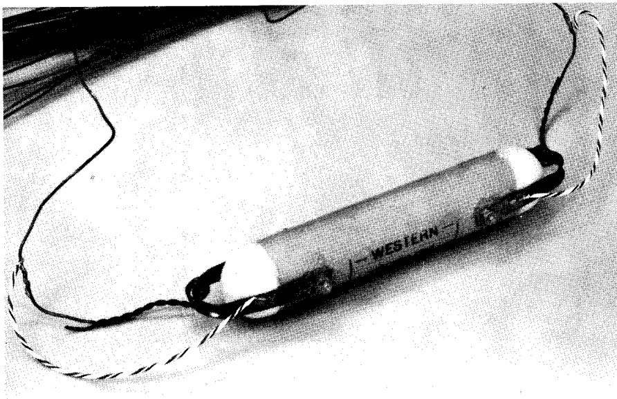
Fig. 6 — Modification of the traps to ensure proper electrical connections between the traps and the wire sections of the dipole. Lock washers have been added to the trap bolts. A coating of clear sealant was added to prevent corrosion where the yokes are mounted to the traps.
