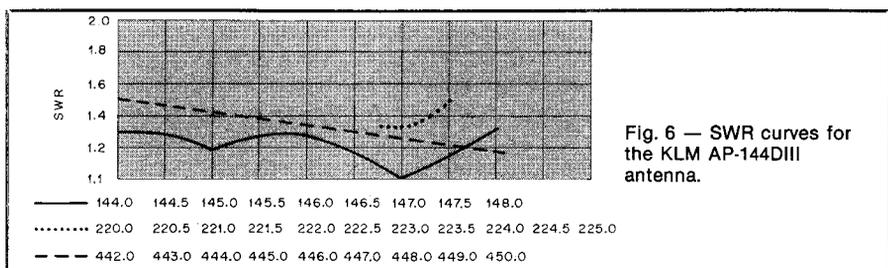
Fig. 6 — SWR curves for the KLM AP-144DIII antenna.
