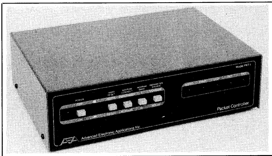
Fig. 2—The AEA PKT-1 comes completely assembled and tested. All that is required is connection to a radio and terminal, and it's ready to go.
