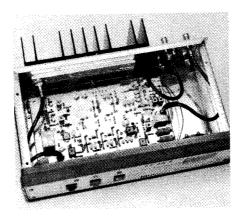
an established West German manufacturer of high-quality VHF and UHF equipment, including transverters and preamplifiers. The subject of this review, a new transverter for the new 902-MHz (33-cm) amateur band, is based on the popular LT 23S 1296-MHz transverter. Anxious to get on 33 cm for the summer, I purchased the LT 33S in May 1986, about 9 months after 902 MHz became available for use in the US. The review unit was from the first production run.
