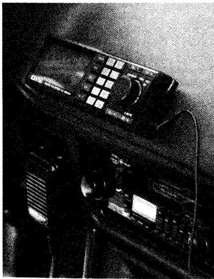
Fig 3—IC-900 remote controller attached to the car dashboard.
