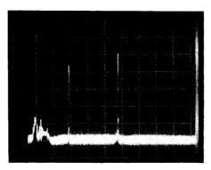
Spectrum Probe display with 21.2- and 50.2-MHz input signals. The dc pip (generated in the Probe) is visible at the second-from-left vertical graticule line. Only the 21.2- and 50.2-MHz signals were applied to the Spectrum Probe for this test; all other visible signals were generated in the Spectrum Probe.
