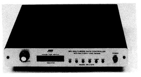
The latest version of the MFJ-1278, due for release in September, has a revised cabinet, gray-scale capability in FAX and SSTV modes, and side-panel adjustable audio levels for both radio ports. Older versions of the '1278 can be upgraded by MFJ to include the features in this latest version.
