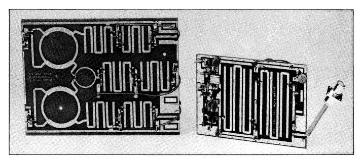
be made. According to John Molnar, WA3ETD, of SHF systems, one of the 10 initial kits also exhibited this problem. Fortunately, his suggested cure of adding a 22-pF chip capacitor between the hairpin filter and ground worked fine, resulting in an oscillation-free, high-gain amplifier chain. This modification is included in current-production kits, although according to Bill Olson, W3HQT, of Down East Microwave, this problem is rare in all but the earliest kits.
