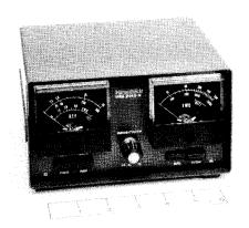
together only by four sets of screws, nuts and washers; it's made such that, if the hardware isn't tight, the meter can come apart when you pick it up by the top cover. Operationally, the meter is a bit clunky; two sets of push-button switches set the power and SWR functions, but their operation isn't quite intuitive. Fortunately, Heath provides a sticker for the cabinet top (or bottom) containing condensed operation instructions.
