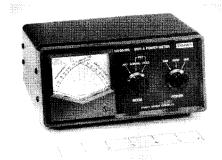
The NS-660PA has a quirk that limits the usefulness of its peak-reading mode: It doesn't indicate reflected power in this mode. So, when you're using the meter in its peak or peak-and-hold mode, the SWR always appears to be 1:1. Only in average-reading mode does the reflected-power needle deflect. The '660PA is more accurate in its peak-and-hold mode than in its peak/no hold mode.
