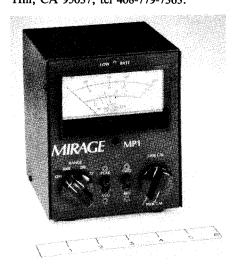
The MP1 is a nice meter to use, but its accuracy isn't great, even though it features an active PEP-indication circuit. Its good features include a flashing low-battery indicator, a large, easy-to-read meter, and
