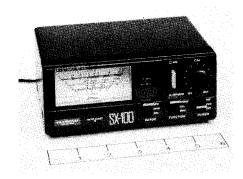
The \$149.95 SX-100 uses a single widedeflection meter movement to indicate forward and reflected power in three ranges (30, 300 and 3000 W). One of the most attractive meters in the bunch, this one uses no active circuitry for peak-power measurements, so its accuracy suffers on low-dutycycle signals. A four-page instruction sheet explains the meter's installation and use in reasonable detail.
