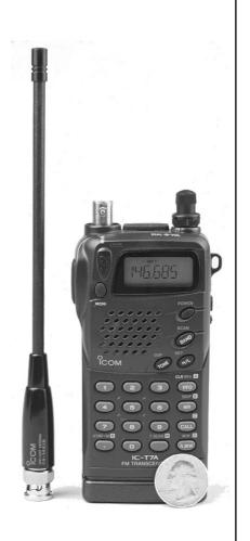
supplied battery, the BP-173 (which also can power the IC-T7A). The BP-173 supplies 9.6 V and is rated at 650 mAh.
