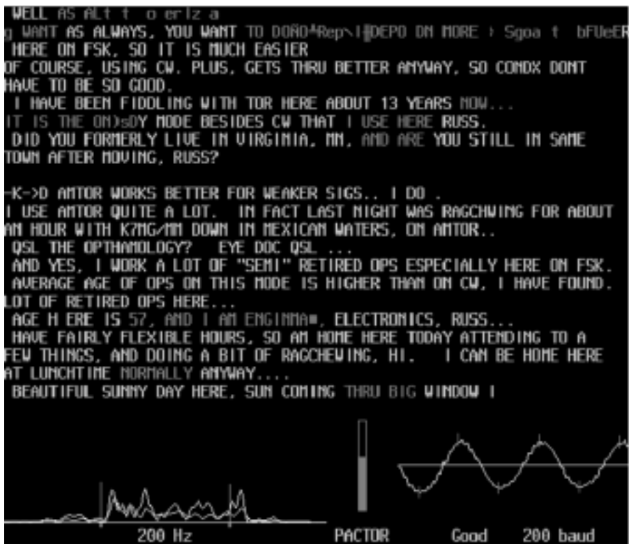
Figure 1—Monitoring PACTOR signals with RITTY 2.0 .
