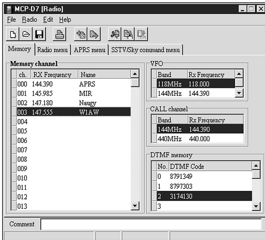
Figure 1—The optional MCP-D7 software and the PG-4W PC Connection Cable allows you to use your PC to program the radio and configure various settings for internal APRS software. You can also use the software to program settings for SSTV operation when using the VC-H1 Visual Communicator. While all of these settings are accessible from the keypad of the radio, the software makes entering data considerably easier.
