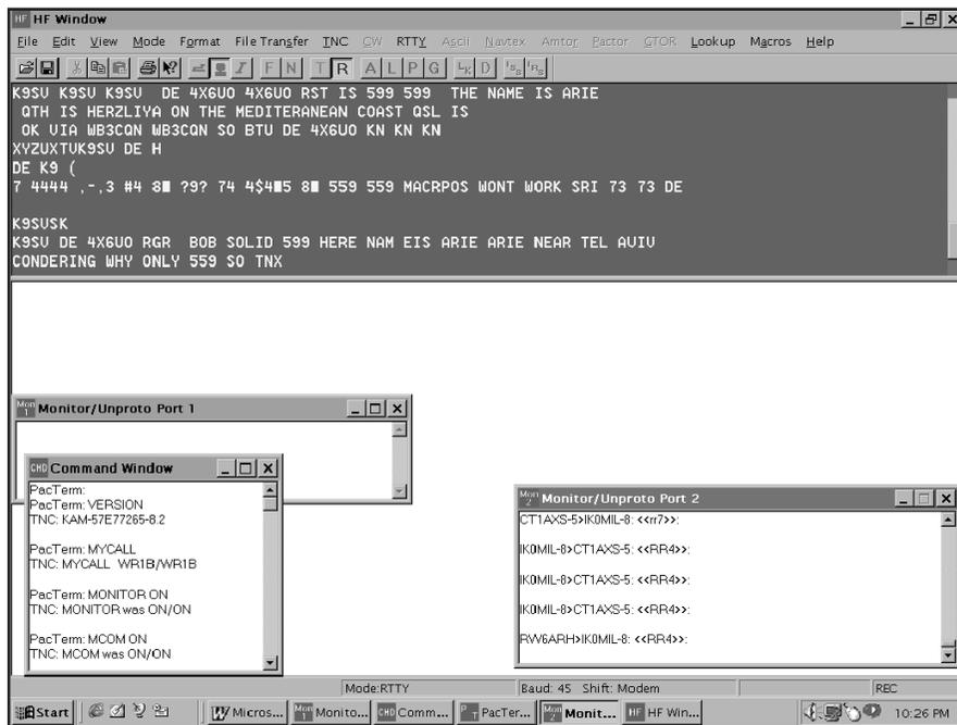
Figure 2—This screen shot shows the *PacTerm 98* screen, with several windows open, monitoring HF and VHF activity.
