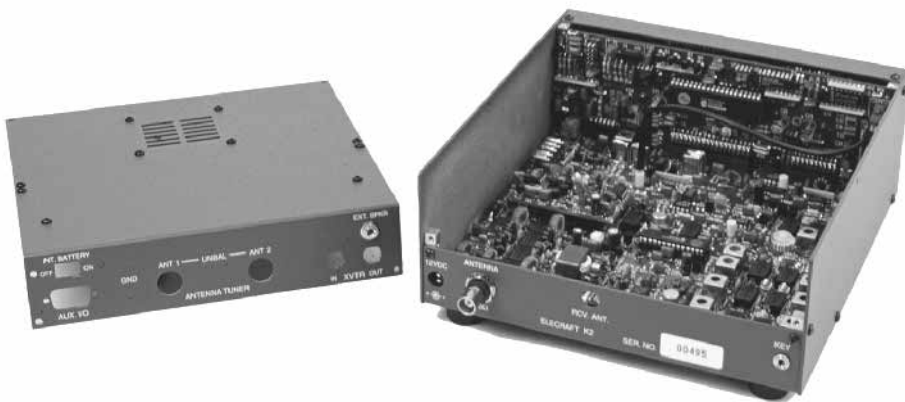
Figure 6—An internal view with the top cover removed. The display and control board plug into the RF board along its front edge. Note the almost total absence of point-to-point wiring. The rear apron is pre-punched for a wide variety of available and proposed optional accessories.
