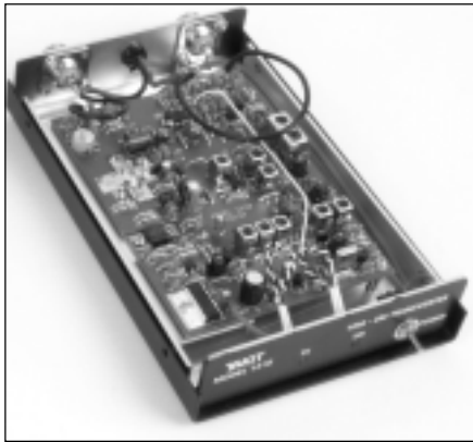
Figure 6—Inside the Ten-Tec 1210 10- to 2-meter transverter. Nearly all the unit's components are mounted on a single 4 × 5½-inch glass-epoxy PC board.
