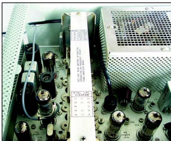
Figure 2—The DDS-2A microprocessor controlled VFO connects to the Collins KMW-2 or KWM-2A via three cables. One plugs into the EXT VFO POWER jack (the black cable on the right side of this photograph) and a second connection is made via a riser inserted between tube V13 and its socket (the gray cable on the left). A third cable, not shown, attaches to the EXT VFO phono jack located on the back panel of the transceiver.
