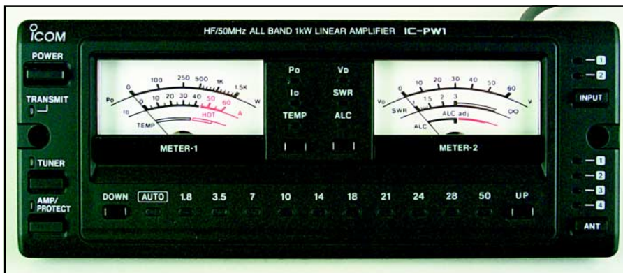
Figure 9—The control panel can be removed from the front of the amplifier's cabinet and relocated up to 10 feet away (the remote cable and a blank cover plate for the amplifier front panel are provided).
