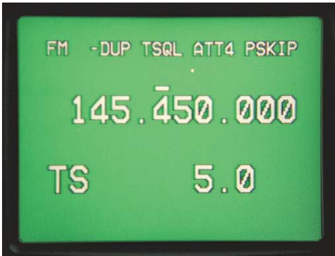
Figure 1—The IC-R3's color TFT main display—available only above 30 MHz—is capable of presenting a tremendous variety of information in several different formats and your choice of eight background colors. This “Simple screen” displays just the bare essentials. The sub LCD shows similar information when the main LCD is off.
