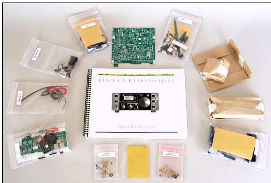
The Elecraft K1 kit as delivered. The majority of the components are presorted into plastic bags, making the inventory and assembly processes considerably more manageable.
