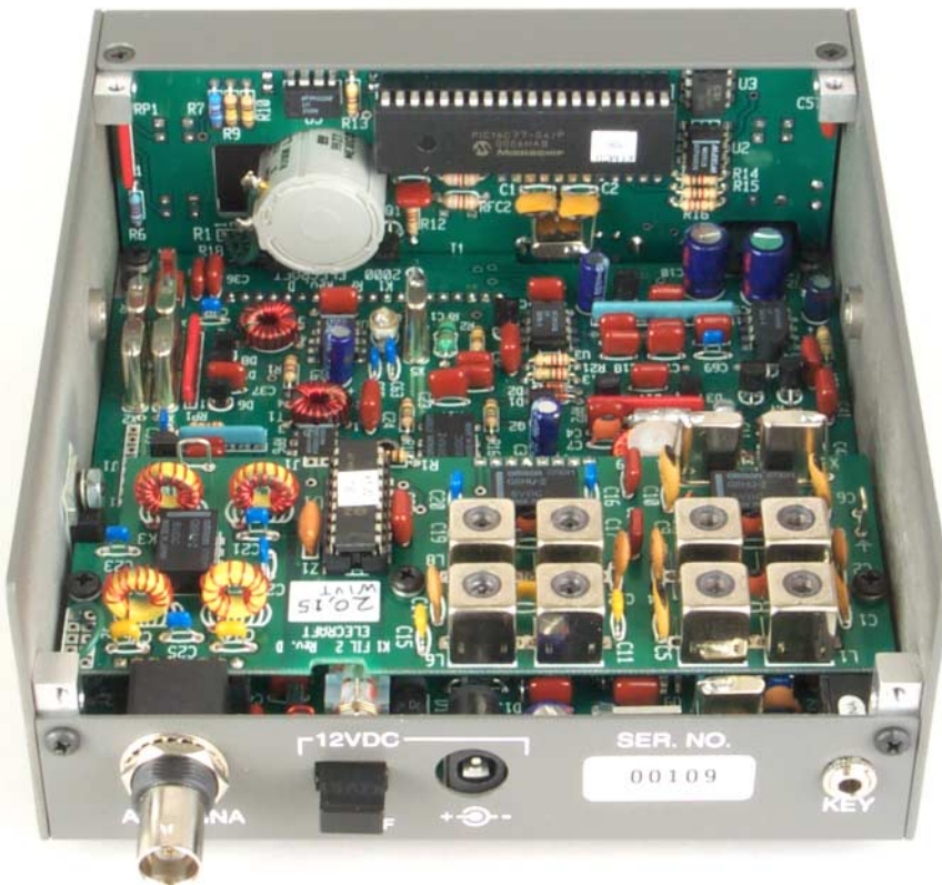
Figure 3—An internal view of W1VT's K1. The Front Panel Board plugs into the main board along its front edge. The Filter Board, which determines the two bands covered by the transceiver, is towards the rear of the enclosure (the foreground in this photo). It's positioned above the RF Board and connects to it through three 8-pin headers. Three small screws secure it in place.
