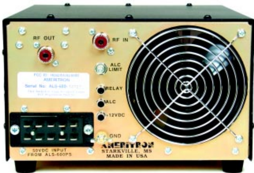
Figure 2—The rear panel of the RF deck.
