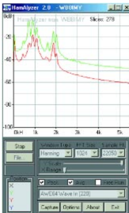
HamAlyzer looks at three PSK31 signals in the peak (top trace) and averaging modes.
