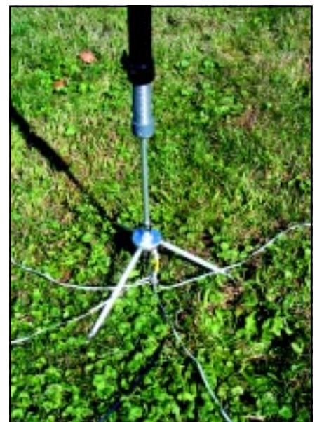
Figure 4 —The MP-1 set up on the optional tripod in a portable application.
