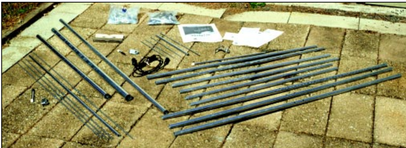
Figure 1—The parts of the A627013S presorted into piles of associated components and ready for assembly.
