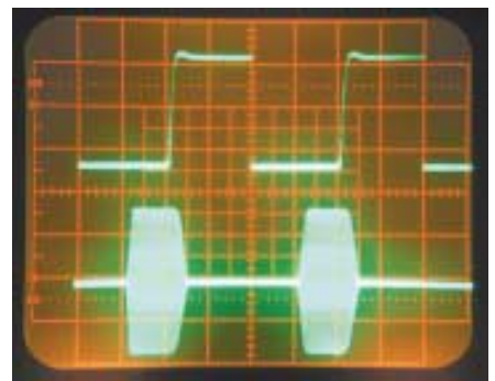
Figure 3—CW keying waveform for the IC-756PROII showing the first two dits in full-break-in (QSK) mode. The equivalent keying speed is 60 WPM. The upper trace is the actual key closure; the lower trace is the RF envelope. Horizontal divisions are 10 ms. The transceiver was being operated at 100 W output at 14.2 MHz. Note that both dits are somewhat shortened. Only the first dit is shortened in semi-break-in mode.
