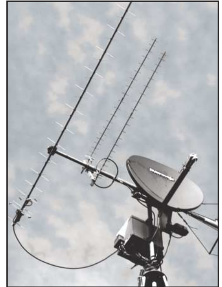
Figure 6—On the air at WD4FAB: two completed 23CM22EXAs in action at the author’s station.
