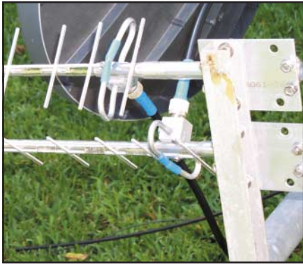
Figure 5—Channel mounting of two 23CM22EXAs for right-hand circular polarization.
