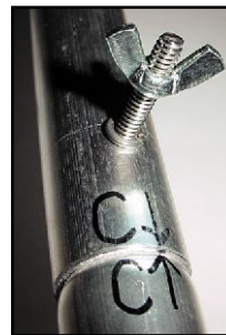
Figure 4—Each joint is clearly labeled. Assembly requires machine screws and finger-tightened wing nuts.
