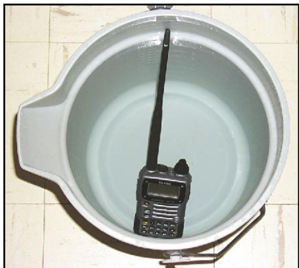
Figure 1—The front panel and front cover of user's manual for the Yaesu VX-7R says the radio is submersible. We put it to the test in the ARRL Lab.
