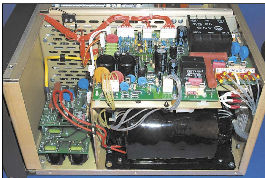
Figure 3—The power supply circuitry inside the ACOM 1000.
