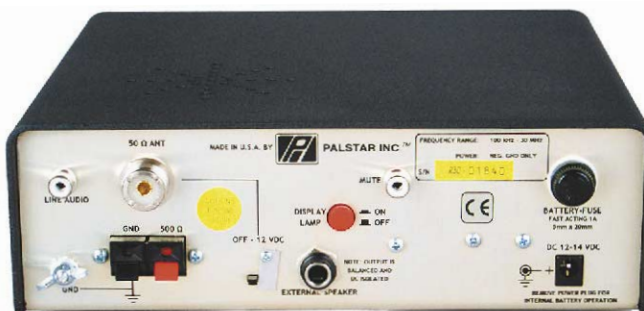
Figure 4—The back panel of the Palstar R30. In addition to the antenna connectors and the audio and control jacks, the display lamp switch is back here. Keep the 12 V dc switch blocked unless you need to send power down the coaxial cable to an active antenna.
