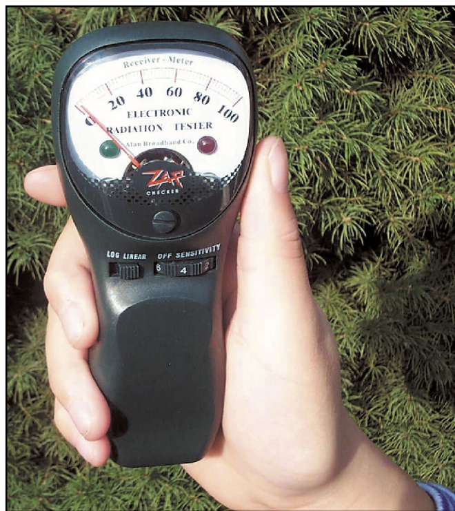
Using the Zapchecker for a back yard fox hunt. The red LED glows when Zapchecker detects a strong signal.
