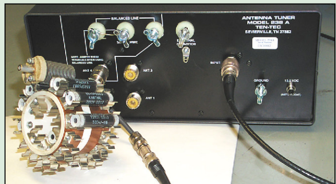
This is a close-up of the parallel load test fixture. The variable capacitor was used to compensate for fixture inductance encountered at some frequencies.
