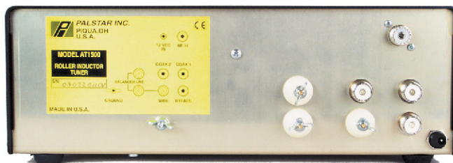
Rear panel connections on the Palstar AT1500CV.
