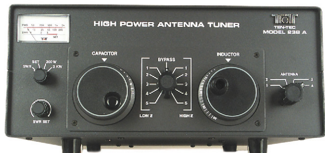
Front panel of the Ten-Tec 238A.
