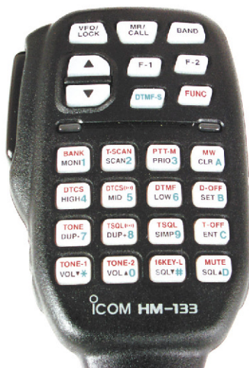
Figure 1—Close-up view of the IC-2720H’s microphone, a control panel in itself. Users who, for some reason, really don’t need a display may plug the microphone directly into the main unit, bypassing the stand-alone control panel.
