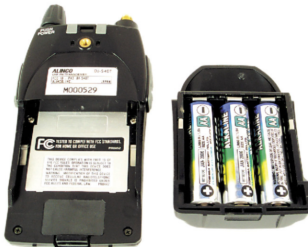
Figure 2—Batteries not included: The DJ-S40T does not come with a rechargeable battery or a charger, although the user may purchase them as optional equipment. Three AA batteries must be provided by the user. Yes, all three go in the same way: negative pole at the bottom; positive at the top. As you can see, the rig is tiny; the battery pack provides a great deal of the radio's volume (as measured in cubic units of length, not dB).
