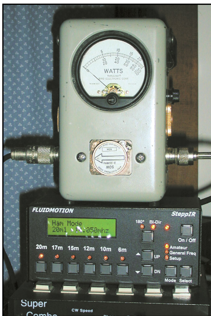
Figure 7—The SteppIR controller and the Bird wattmeter used during testing.
