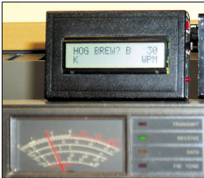
Figure 4 (left)—Is the sender talking about activities at W5YM, the station at the University of Arkansas? No! The sender didn't leave enough space between the M and the E in home brew . This illustrates the limitations of the MFJ-461—or nearly any other firmware or software Morse reader—when copying imperfect code. Still, it does a pretty credible job at 30 WPM. Notice that the K in “BK” is scrolled to the next line.
