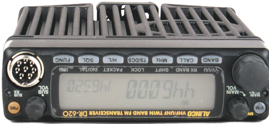
Figure 5—(Top) Is this a defect? Did Alinco manufacture this unit of the DR-620T upside down? No, not at all. Alinco allows the user to decide whether she wants the speaker facing up or facing down by rotating the front panel 180 degrees. (Right) As you can see, in this configuration, the speaker is at the bottom of the radio, ideal for mounting just under a shelf or dashboard.
