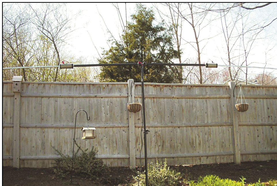
The Buddipole set up in my back yard and tuned for 20 meters.
