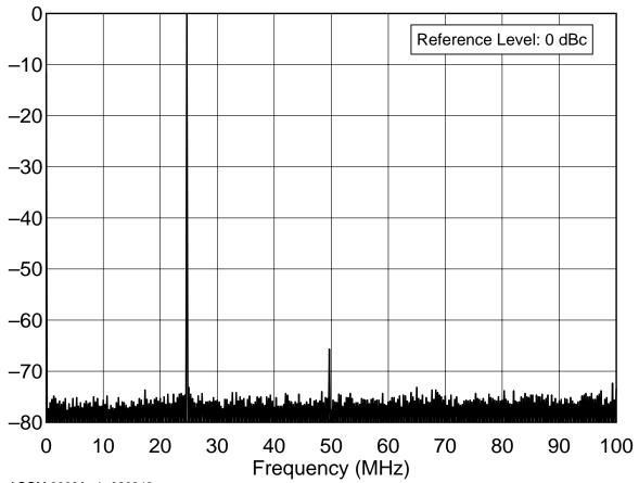
ACOM 2000A s/n 990346 24.9 MHz Band, Spectral Purity, 1500 W C:\!TESTS\ACOM\2000AS12.TXT
