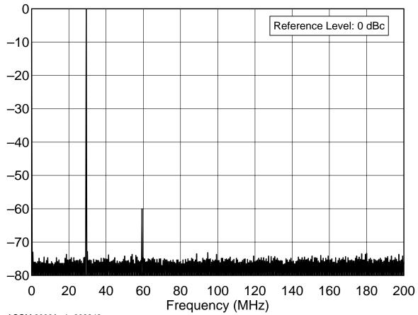
ACOM 2000A s/n 990346 28.0 MHz Band, Spectral Purity, 1500 W C:\!TESTS\ACOM\2000AS10.TXT
