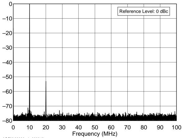
ACOM 2000A s/n 990346 10.1 MHz Band, Spectral Purity, 200 W C:\!TESTS\ACOM\2000AS30.TXT
