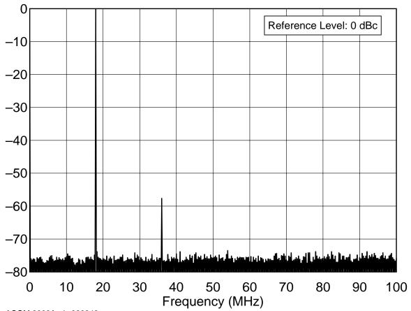
ACOM 2000A s/n 990346 18.1 MHz Band, Spectral Purity, 1500 W C:\!TESTS\ACOM\2000AS17.TXT
