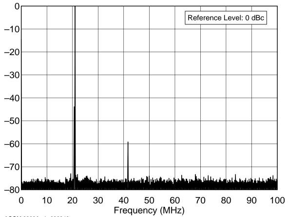
ACOM 2000A s/n 990346 21.0 MHz Band, Spectral Purity, 1500 W C:\!TESTS\ACOM\2000AS15.TXT
