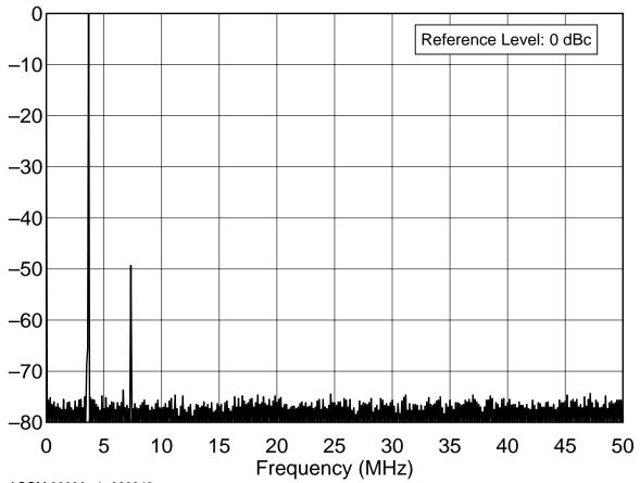
ACOM 2000A s/n 990346 3.5 MHz Band, Spectral Purity, 1500 W C:\!TESTS\ACOM\2000AS80.TXT
