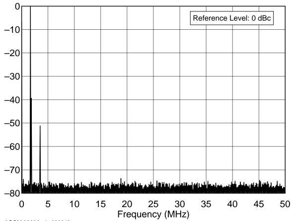
ACOM 2000A s/n 990346 1.8 MHz Band, Spectral Purity, 1500 W C:\!TESTS\ACOM\2000ASLO.TXT
