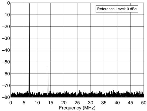
ACOM 2000A s/n 990346 7.0 MHz Band, Spectral Purity, 1500 W C:\!TESTS\ACOM\2000AS40.TXT
