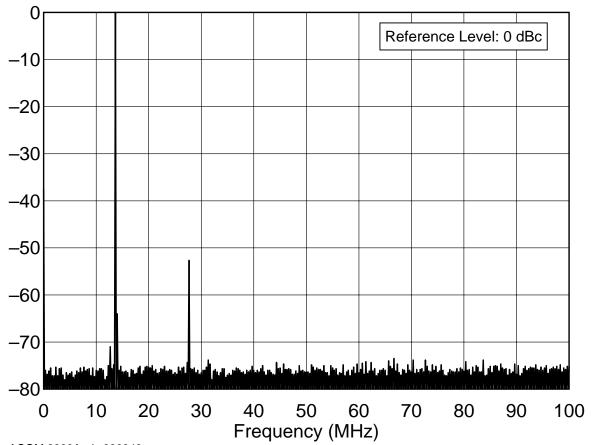
ACOM 2000A s/n 990346 14.0 MHz Band, Spectral Purity, 1500 W C:\!TESTS\ACOM\2000AS20.TXT
