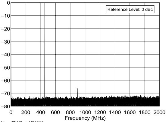
Yaesu FT-90R s/n 9F050205 420.0 MHz Band, Spectral Purity, 35 W C:\MYDOCU~1\PRODREV\TESTDATA\YAESU\FT90R\FT90RS70.TXT
