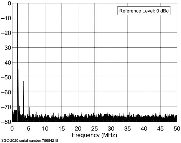
1.8 MHz Band, Spectral Purity, 20 W F:\SHARED\PROD\_REV\TESTS\SGC2020.2ND\SGC20SLO.TXT
