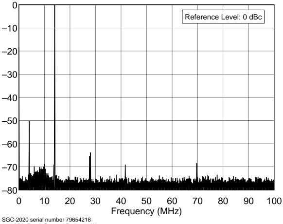
14.0 MHz Band, Spectral Purity, 20 W F:\SHARED\PROD\_REV\TESTS\SGC2020.2ND\SGC20S20.TXT
