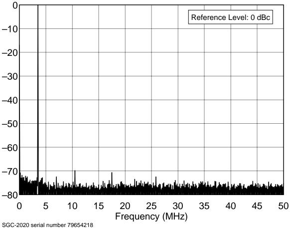
3.5 MHz Band, Spectral Purity, 20 W F:\SHARED\PROD\_REV\TESTS\SGC2020.2ND\SGC20S80.TXT
