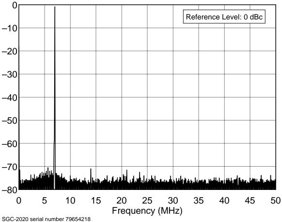
7.0 MHz Band, Spectral Purity, 20 W F:\SHARED\PROD\_REV\TESTS\SGC2020.2ND\SGC20S40.TXT
