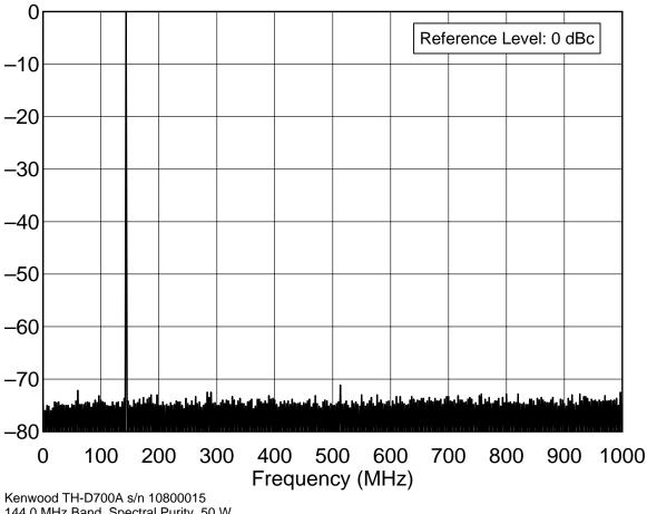
144.0 MHz Band, Spectral Purity, 50 W C:\!TESTS\TH-D700A\TH700S2M.TXT
