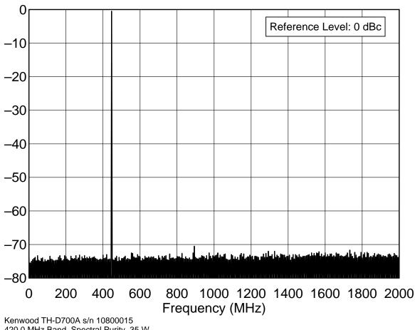
420.0 MHz Band, Spectral Purity, 35 W C:\!TESTS\TH-D700A\TH700S70.TXT
