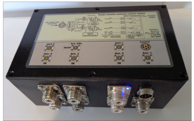
Photo 3A3. Top-down view of the antenna switch, highlighting placement of all the sockets on one side of the diecast box.
