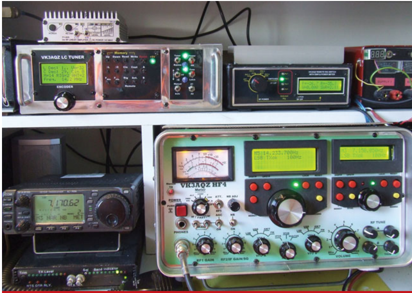
The ATU and antenna switch in use in my shack.
