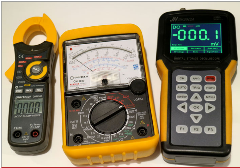
Multimeters come in many styles. On the right is a DMM with 10 MHz oscilloscope, as well. Don't dismiss analogue multimeters, they can be extremely useful when measuring fluctuating signals. The clamp meter at left can measure current without 'opening' the circuit under test.
