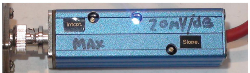
A metal enclosure is essential for the instrument's RF head shielding.
