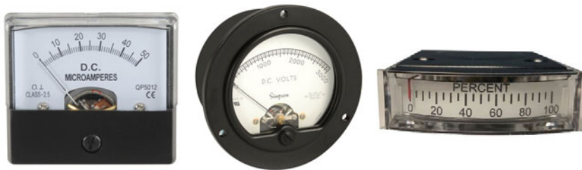
Figure 1. Analogue panel meters come in a variety styles. These are moving coil meters having a pointer that moves over a scale to show a value in response to current flow.
