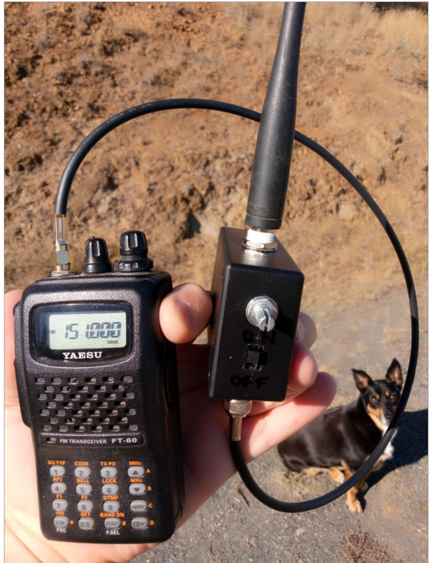
Figure 12: Testing the unit. It's tuned to 151 MHz here, 4 MHz above the 147 MHz signal from VK5RAD.
