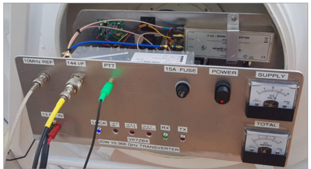
Photo 2: Richard VK7ZBX's 20 W 10 GHz transverter mounted on the rear of the 1.8 m dish.
