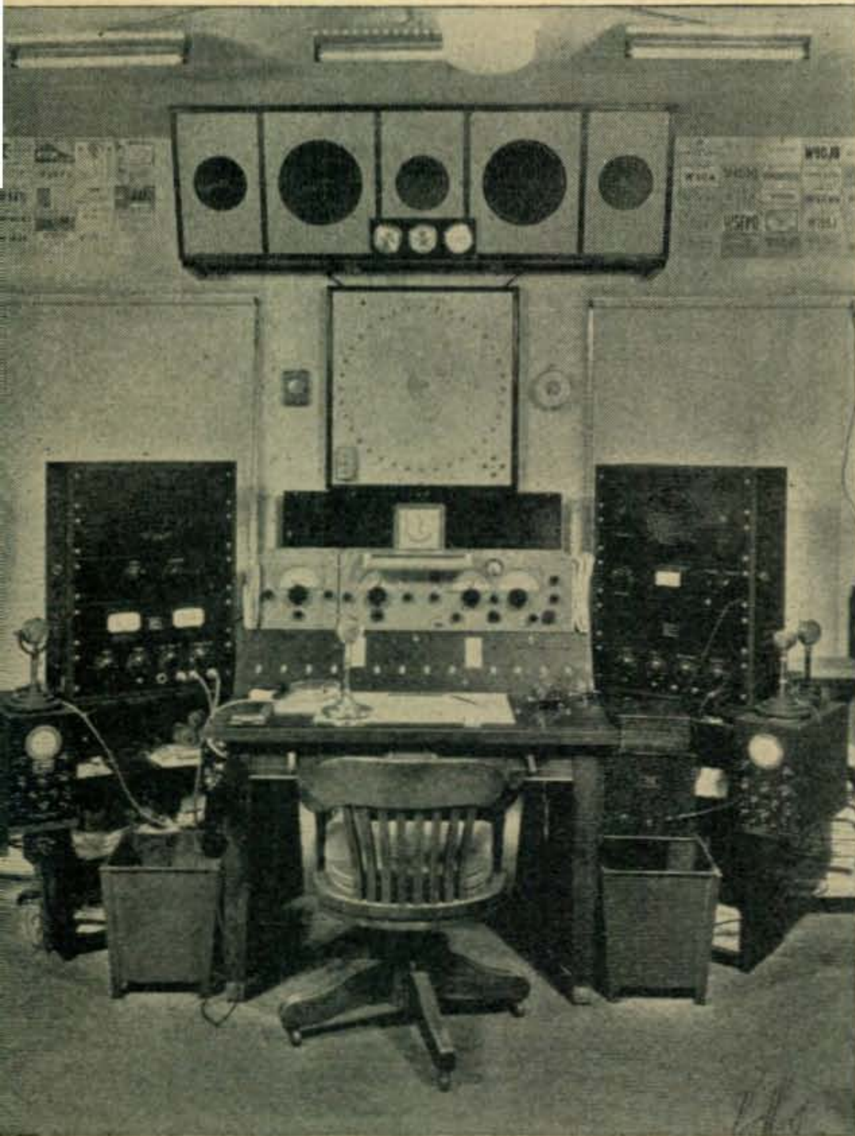
Fig. 4. Control desk at W4EDD. The dots around the framed map are lamps showing the direction the motor-driven rotary antenna is beamed
