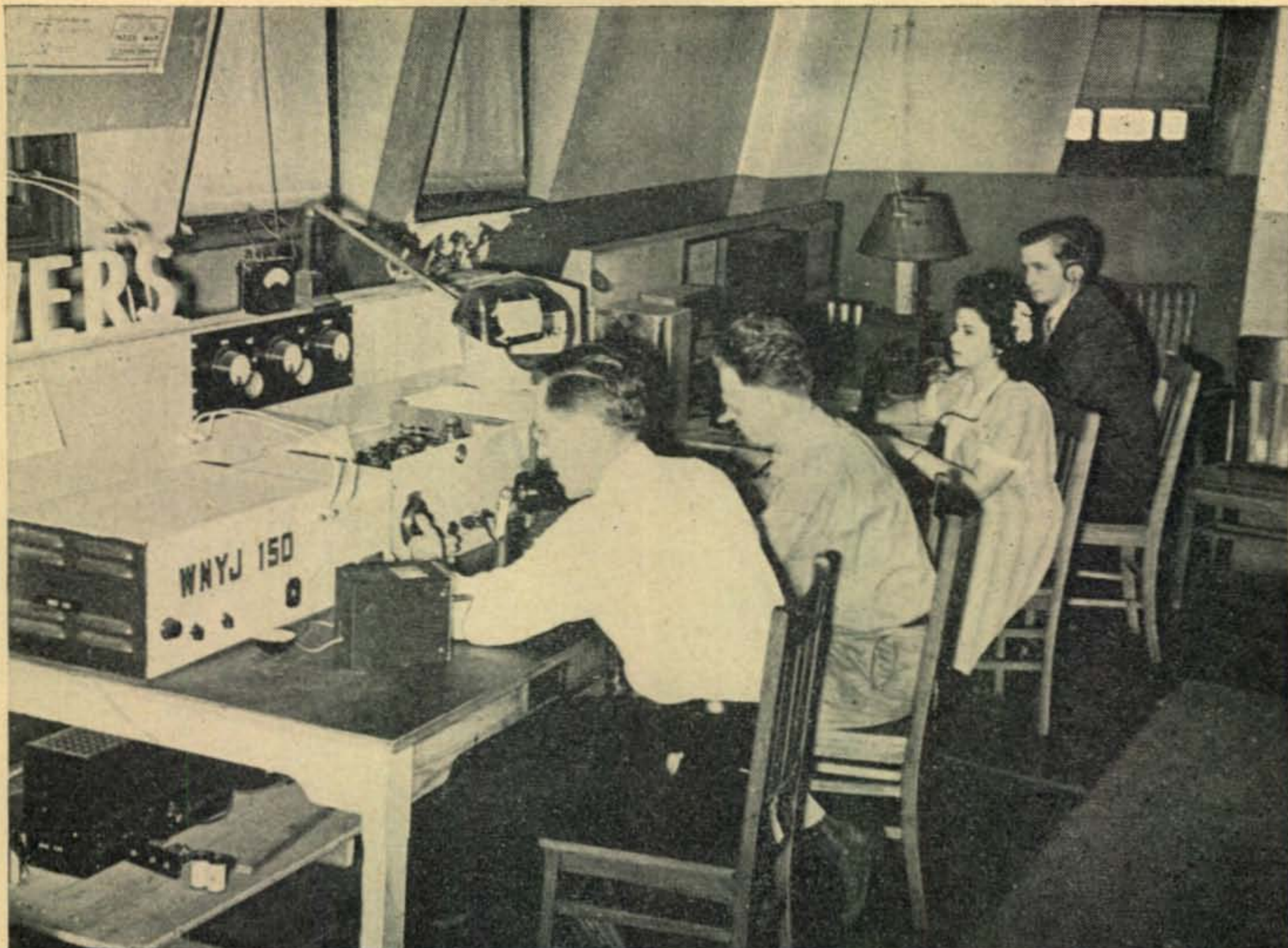
Fig. 5 (above). View of City Control, WNYJ-150, showing the main transmitter at the left; the main receiver, an AM-FM superhet, in front of the Radio Aide speaking into the mike; WNYJ-280 is in front of Chief Electrician E. Lussier. A third receiver is on a third table to the left of WNYJ-150 (not in photo). Below, schematic of transmitter-receiver
