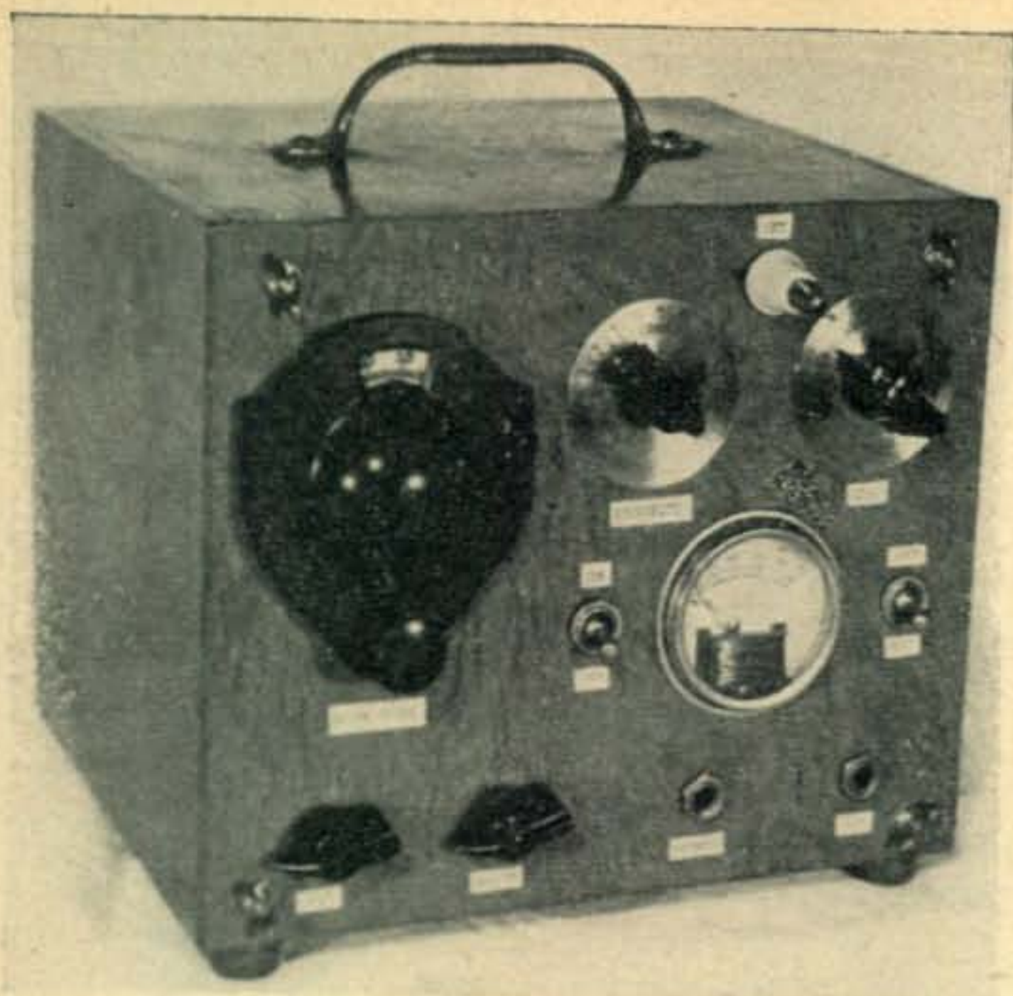
The complete transmitter-receiver unit with batteries enclosed — ten pounds of two-way radio, with a potential long-distance range, in a case 9" wide, 7½" high and 7½" deep
