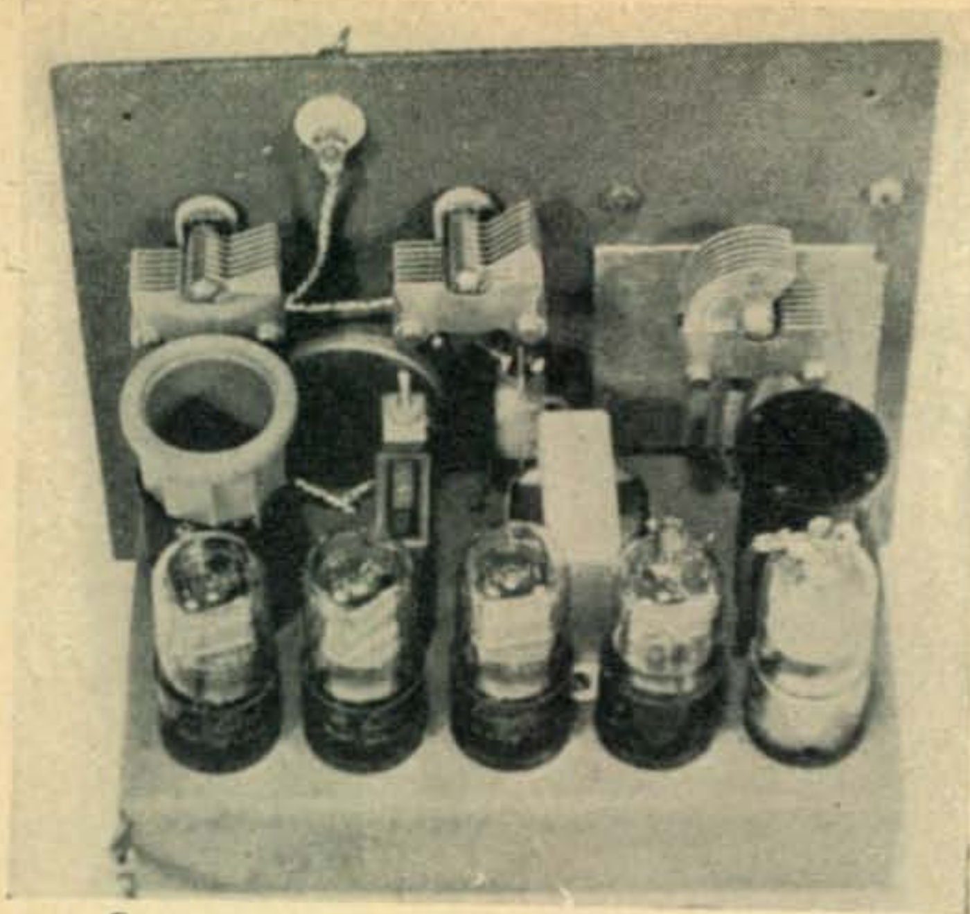
Transmitting coil, L_1 , is behind output condenser on extreme left. Crystal, with shield removed, is next to it. Audio transformer is in the center with the receiving coil unit, L_2 , on the right
