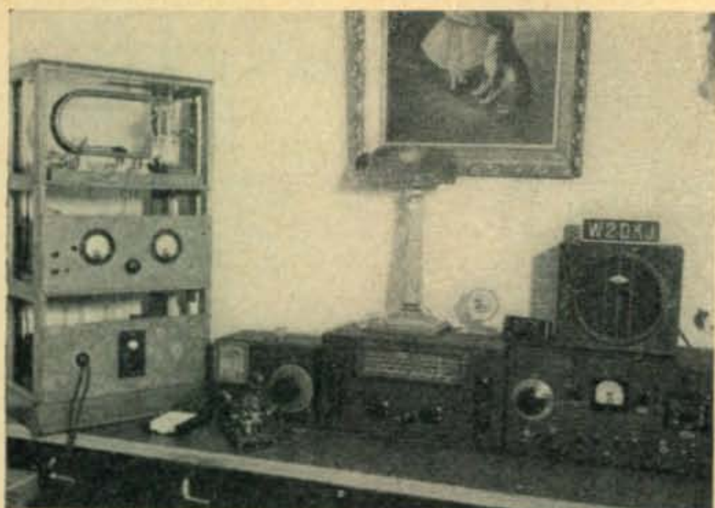
One of the author's pre-war rigs. The transmitter on the left and the National "1-10" receiver were operated on 2½ meters with antennas similar to those described in the article
