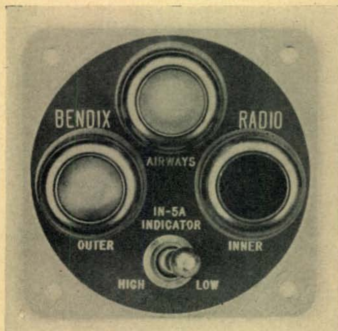
75 mc indicator lamp instrument —Courtesy Aero Digest
