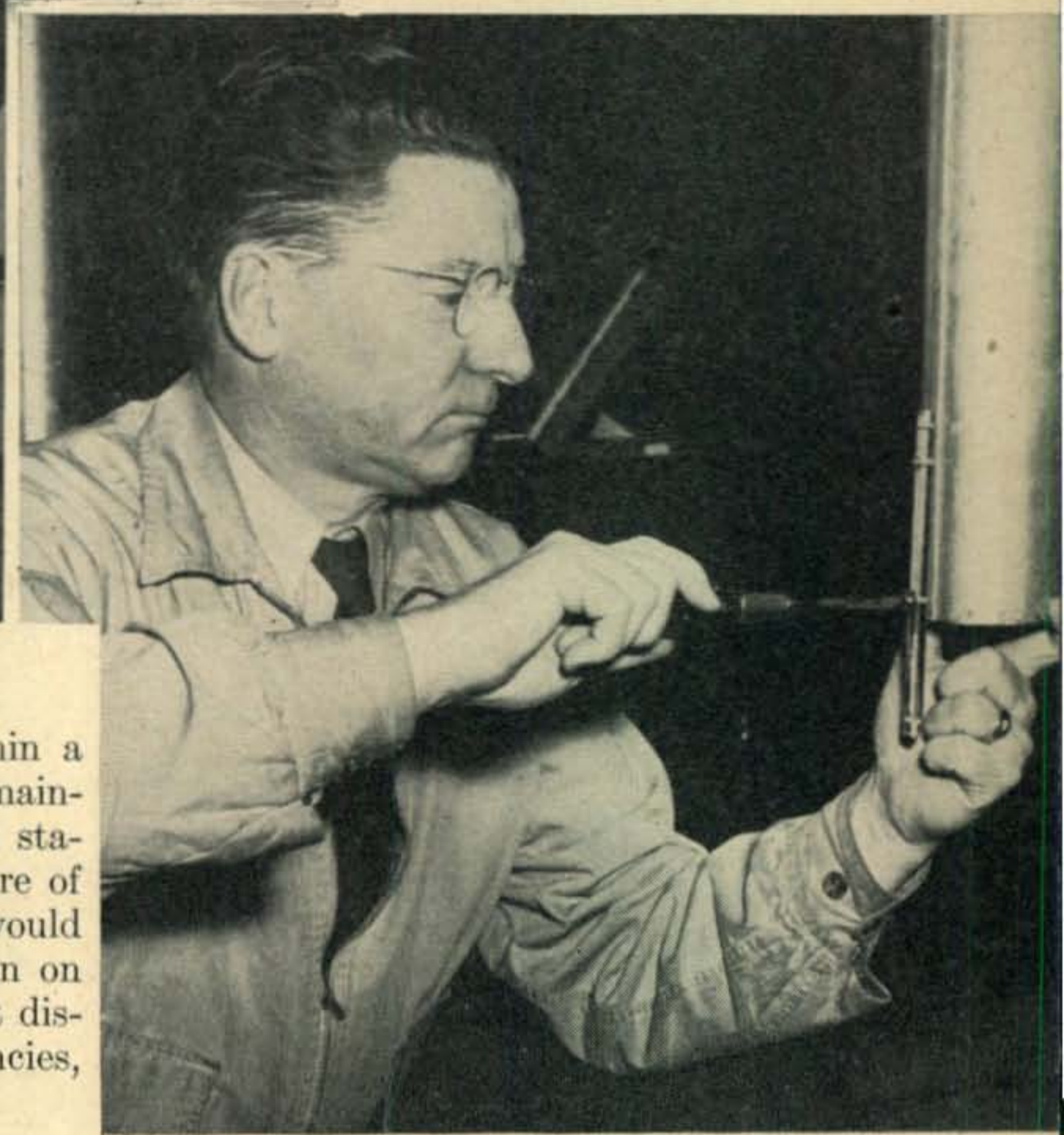
(below). Affixing strips for feeder connection on the lower ends of the proper antenna
