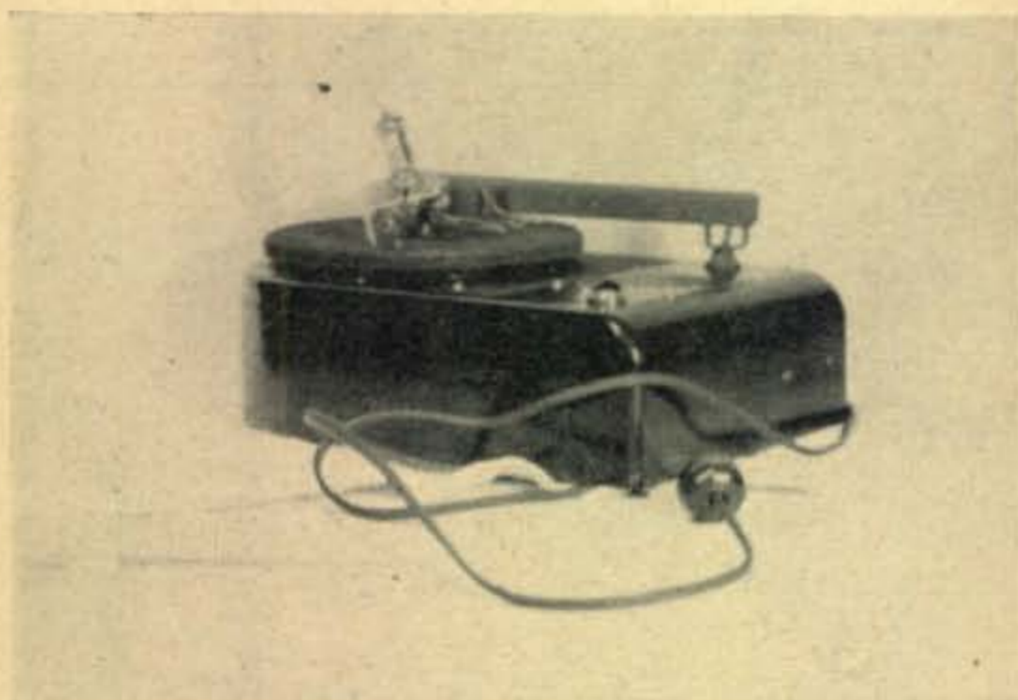
Fig. 4. The completed record player, with the 3S4 amplifier on the turntable. When used, this is mounted inside the case, to the right of the 117L7GT
