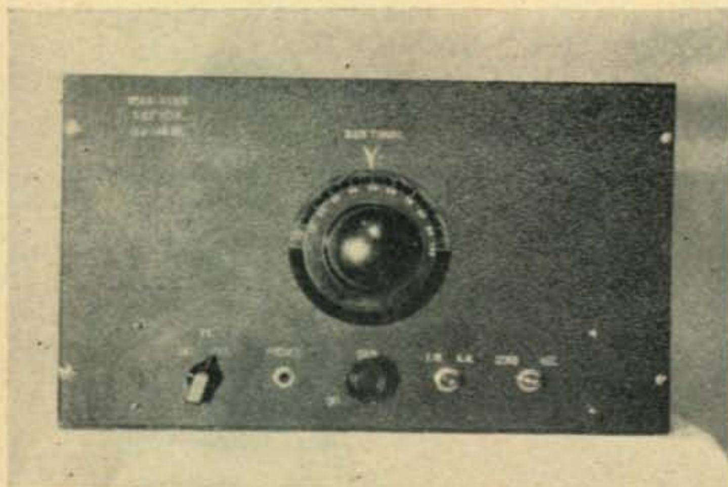
The finished job. Professional lettering was done with a regular rubber stamp and white paint
