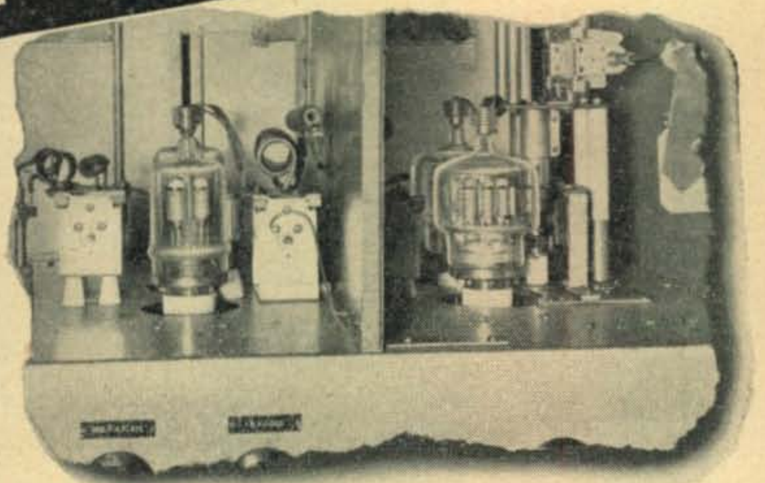
Eimac 152-T's are used in the modulated stage and 304-T's in the first Class B linear amplifier of the video transmitter.
