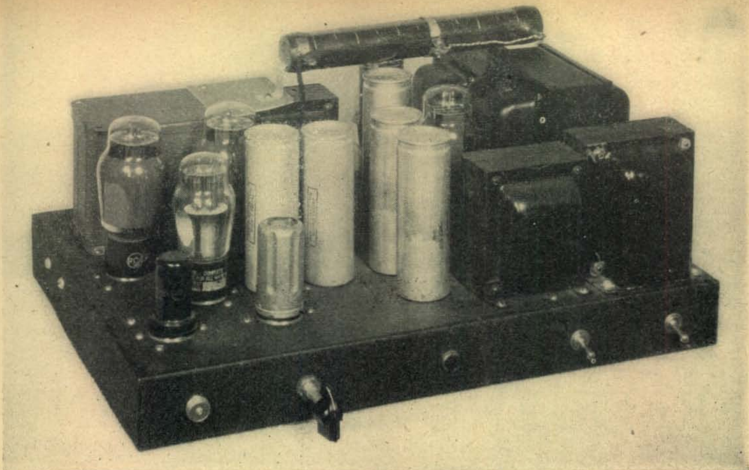
Fig. 5. The modulators, speech amplifier and power supplies. The large resistor lowers voltages for test purposes had convinced us that some amount of QSY would be necessary.
