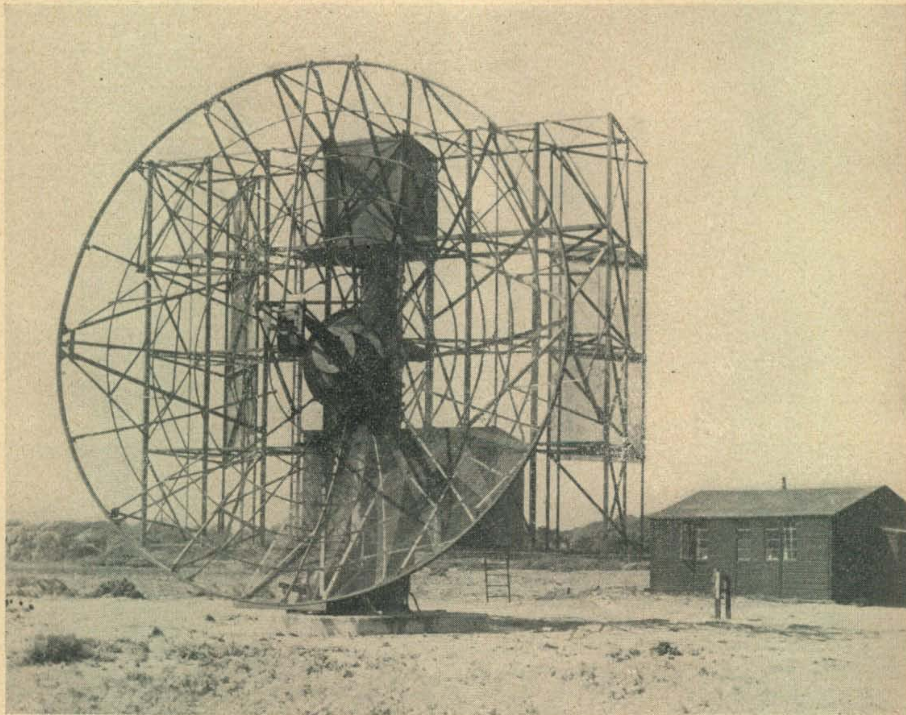
Fighter Direction aerial system for "GCI" (Ground Controlled Interception). The paraboloid is 35 feet in diameter, and the cabin, mounted on the aerial structure, houses both transmitter and receiver
