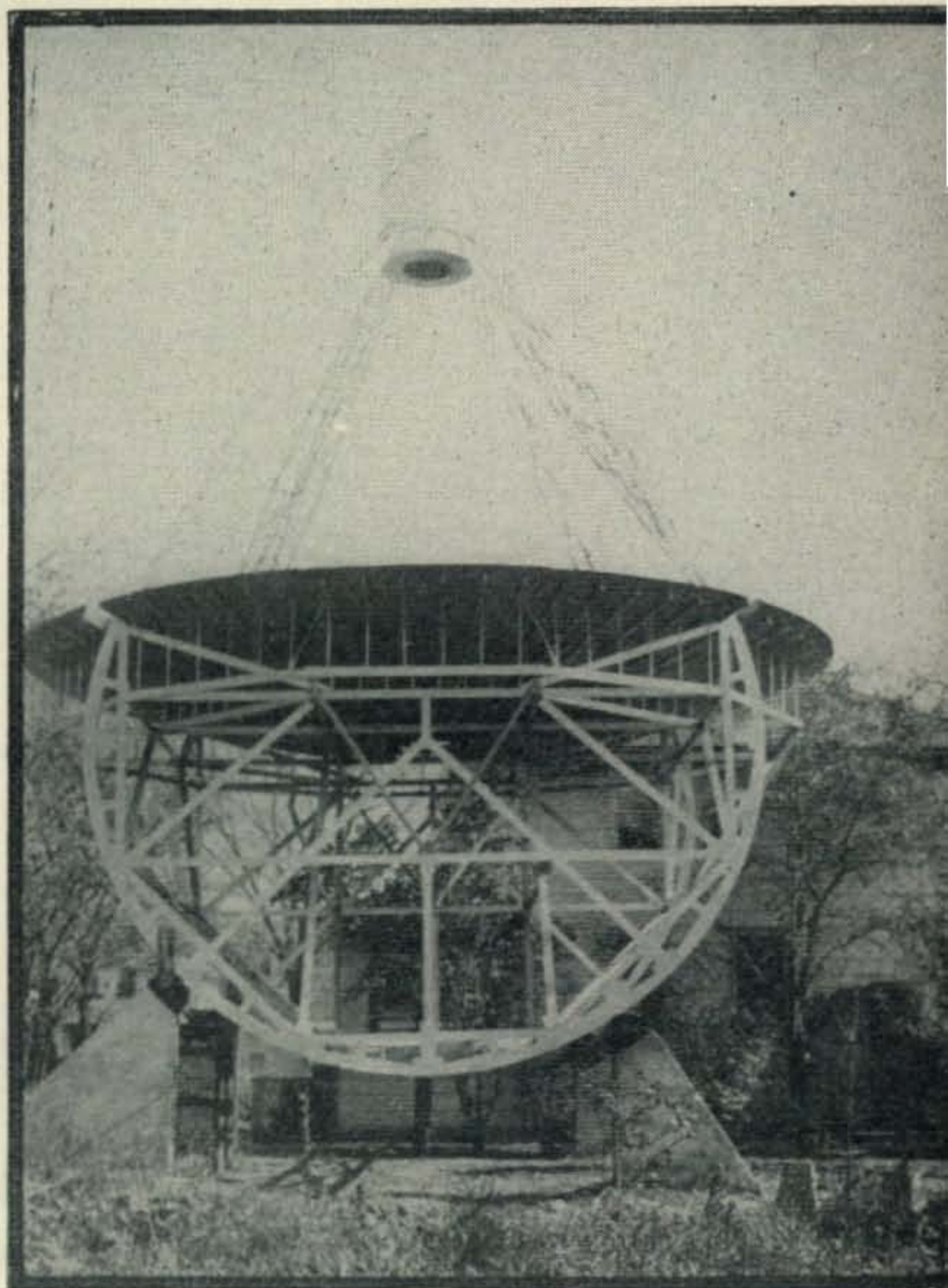
Fig. 2. The W9GFZ reflector for listening in on the cosmic static on 160 mc. It is an example of top-notch amateur experimental work
