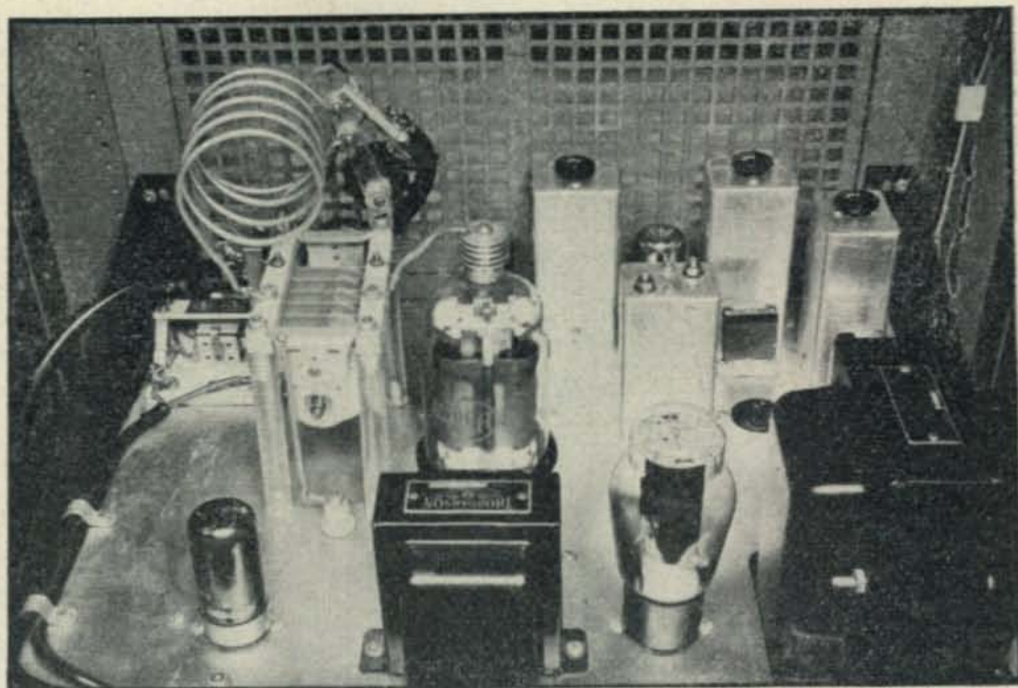
R-F exciter and amplifier showing layout of low voltage power supply, exciter coils, and final amplifier
