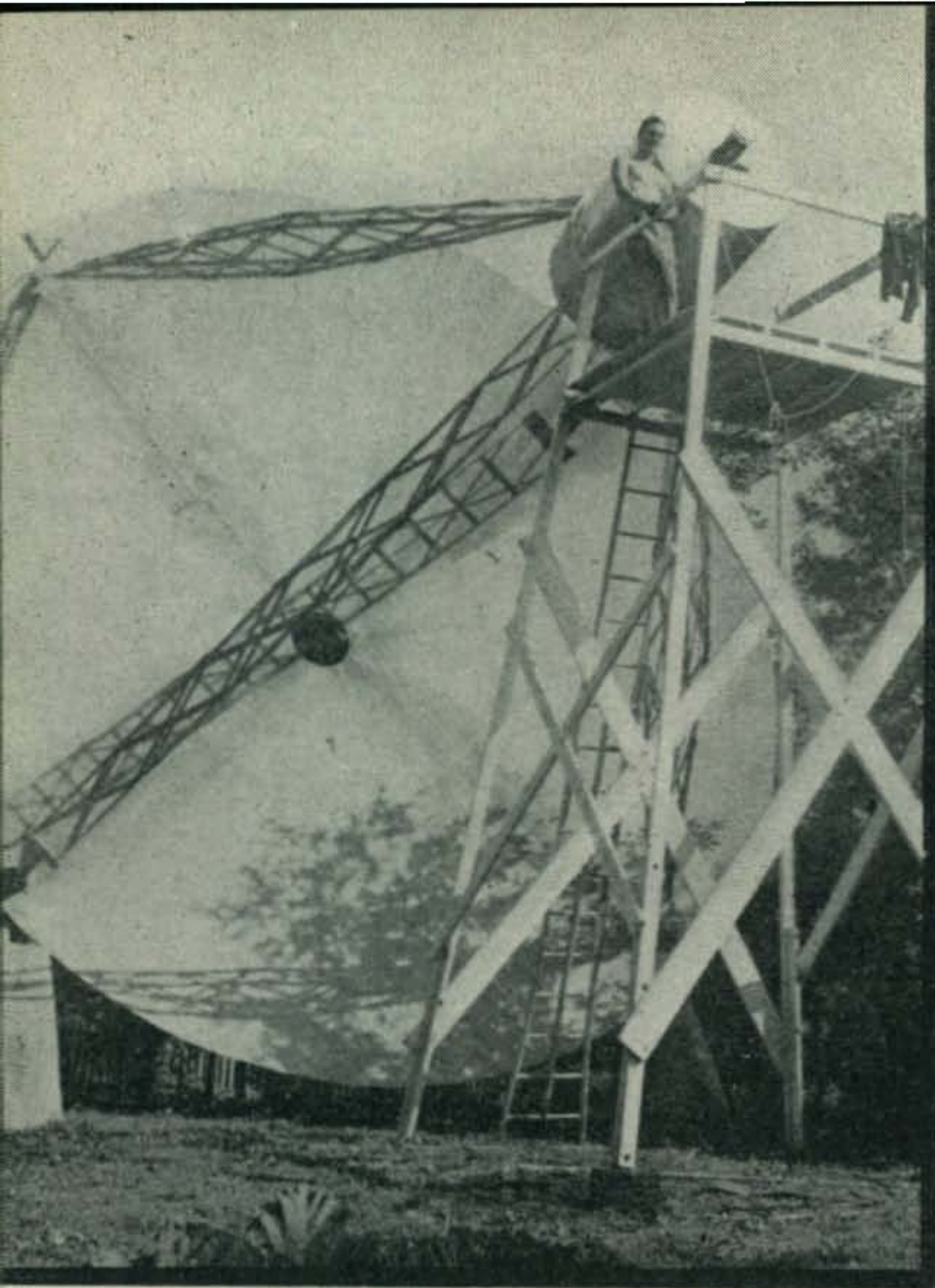
Fig. 3. W9GFZ's parabolic reflector measures 31 feet in diameter and has a focal length of 20 feet. The receiver is mounted in the oil can affair at focus
