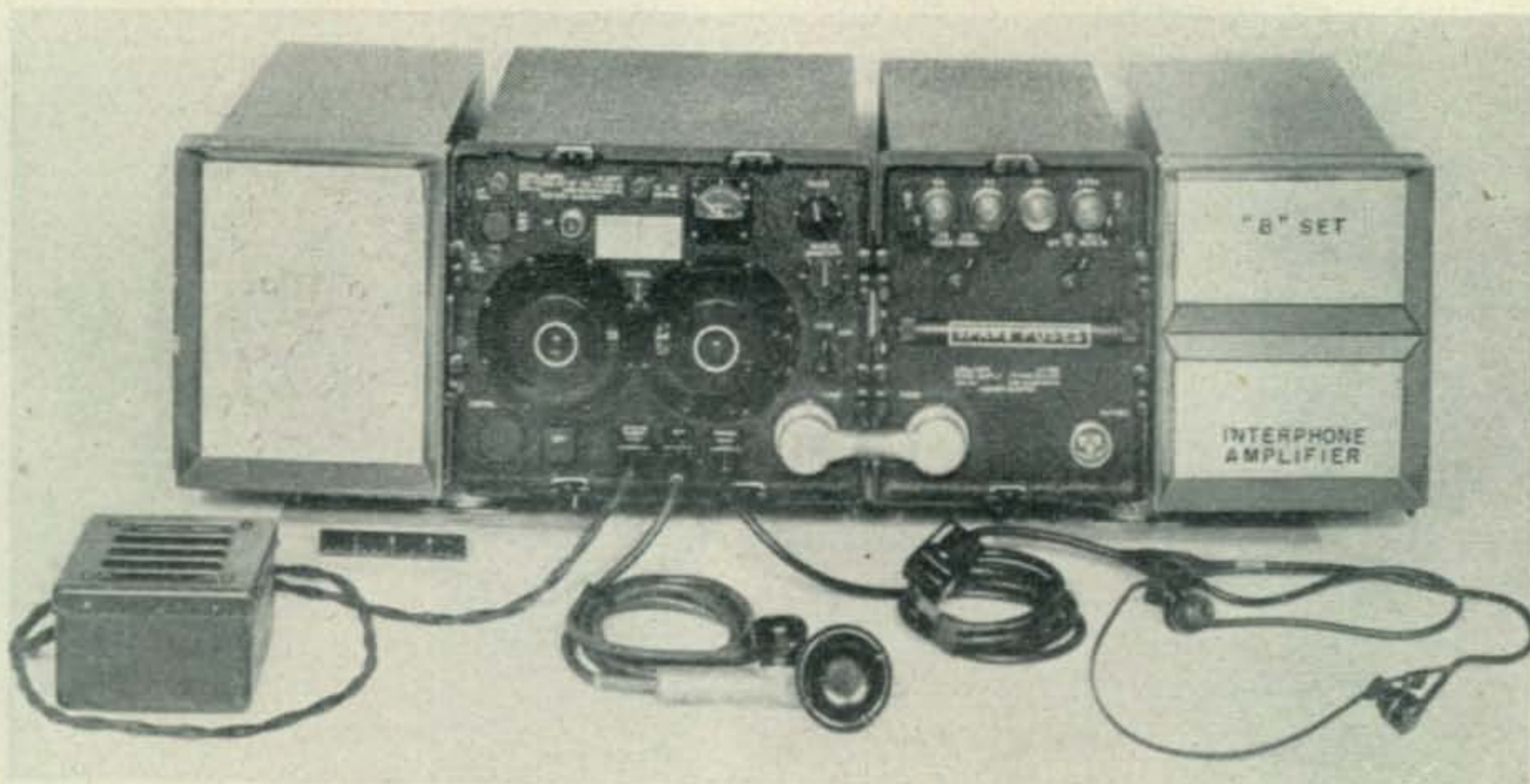
Variations of this RT-67(XC-1)GRC-5 frequency-modulated transmitter-receiver (vibrator power supply) will operate on the FM portions of the 6 and 10-meter bands
