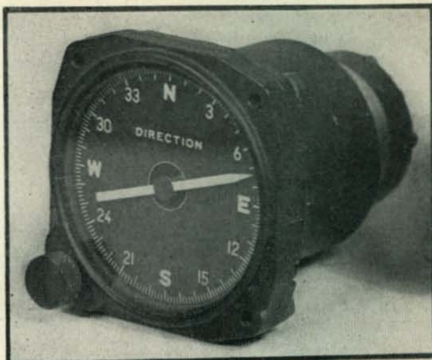
Direction indicator at W1KVV consists of a 1F selsyn motor mounted in a aviation course indicator case
