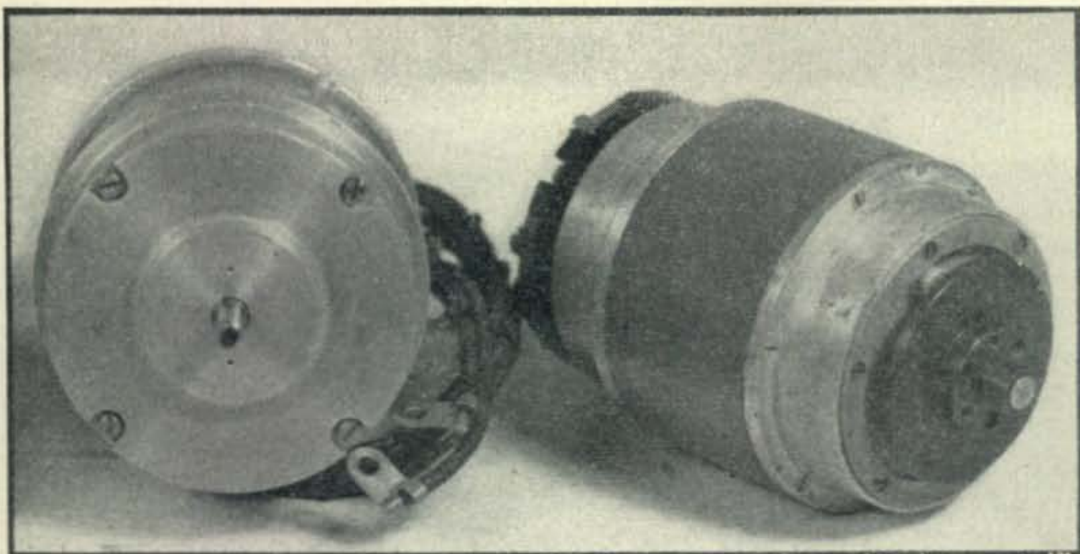
A selsyn generator and motor, size 5, made by two different manufacturers and used in W1KVV's indicating system
