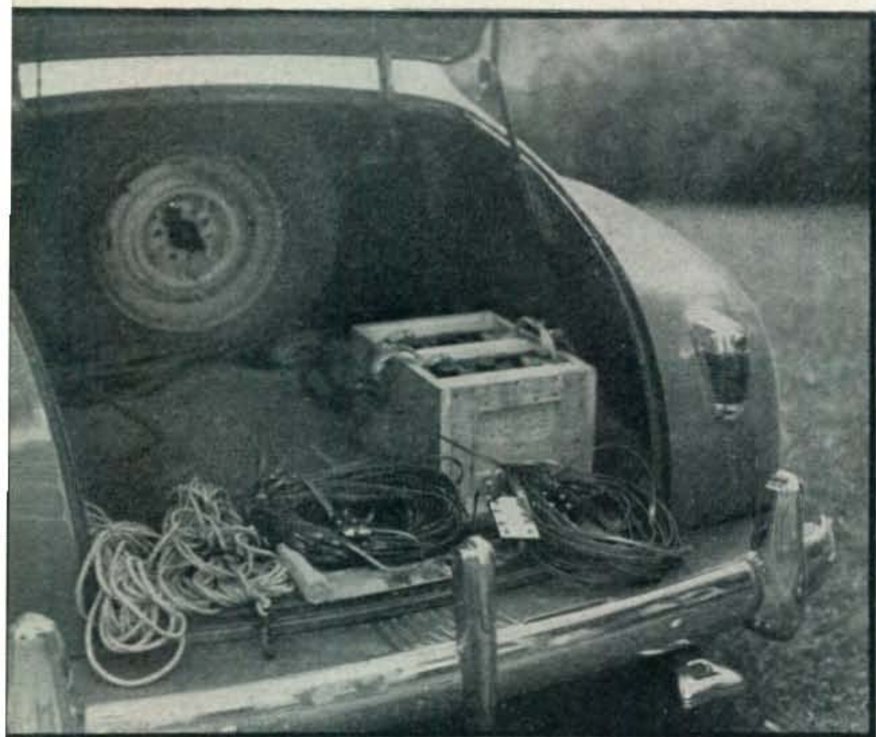
Two 120 amp batteries are used to drive the motor generator set for the SCR-284A. The antenna is coiled in the foreground and is a $6.50 folded dipole. The hemp rope and sash weight are the necessities for raising the antenna above ground.
