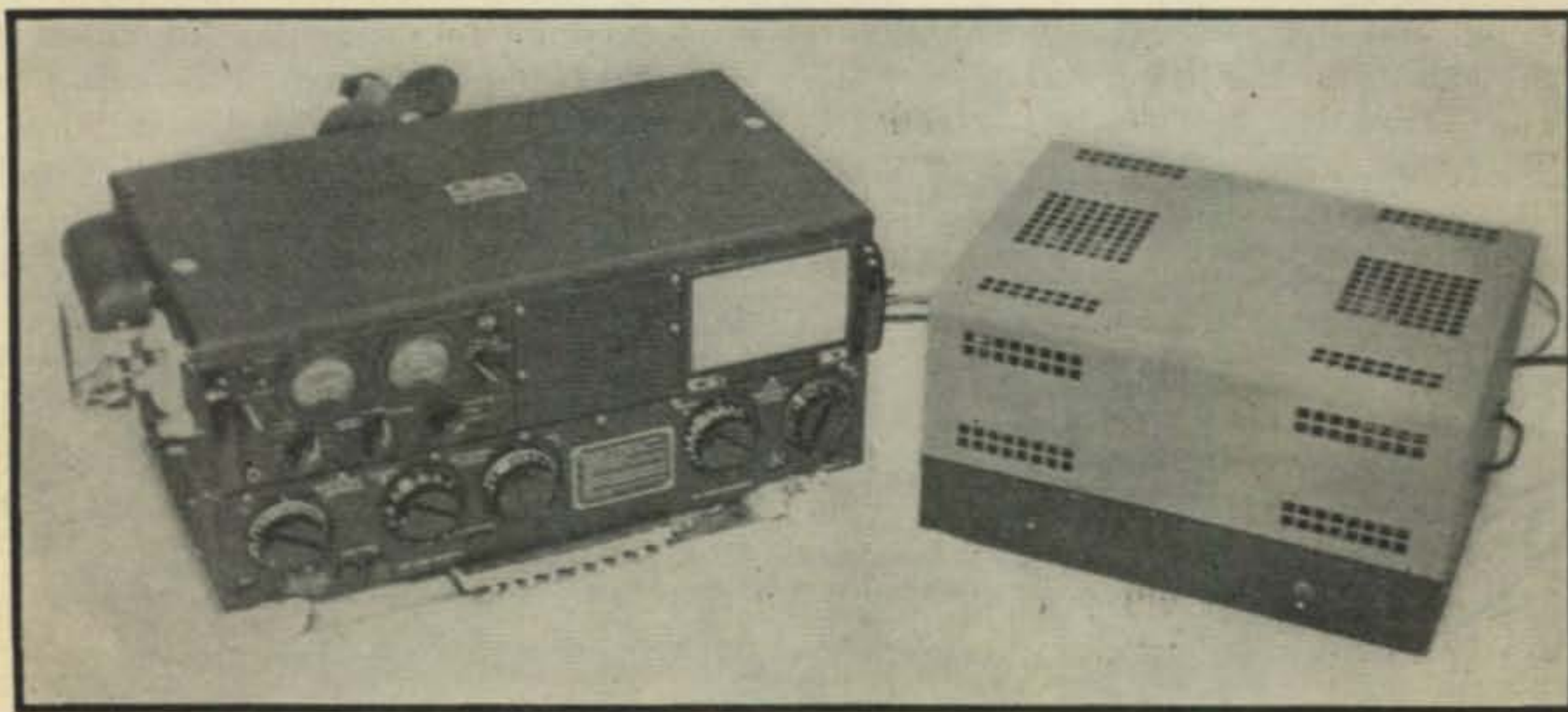
The ART/13 with a-c power supply. Equal in size to the average communications receiver, this aircraft transmitter is rated at 200 watts output on phone and c.w. with automatic selection of 11 frequencies on any band from 80 to 10 meters after conversion.
