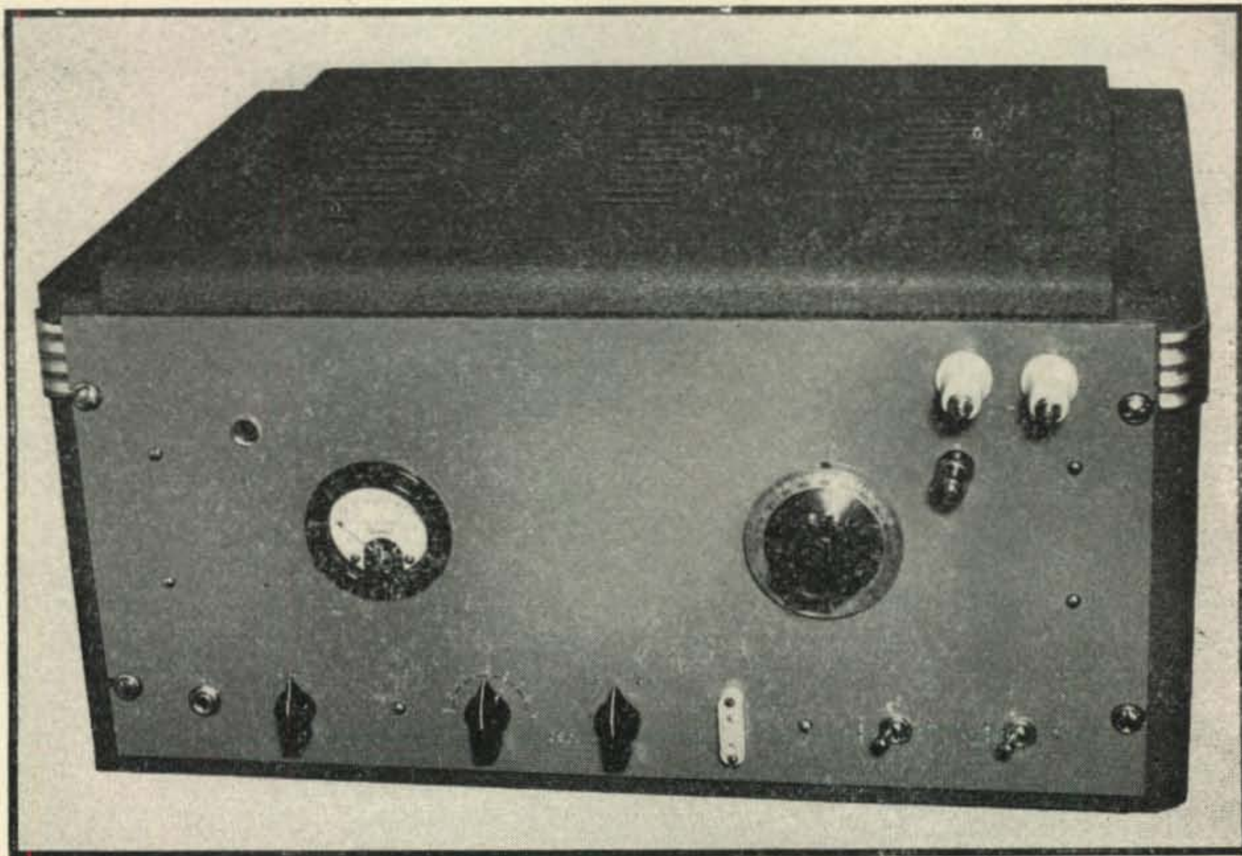
Front view of 60 watt, plate-modulated 807 rig.
