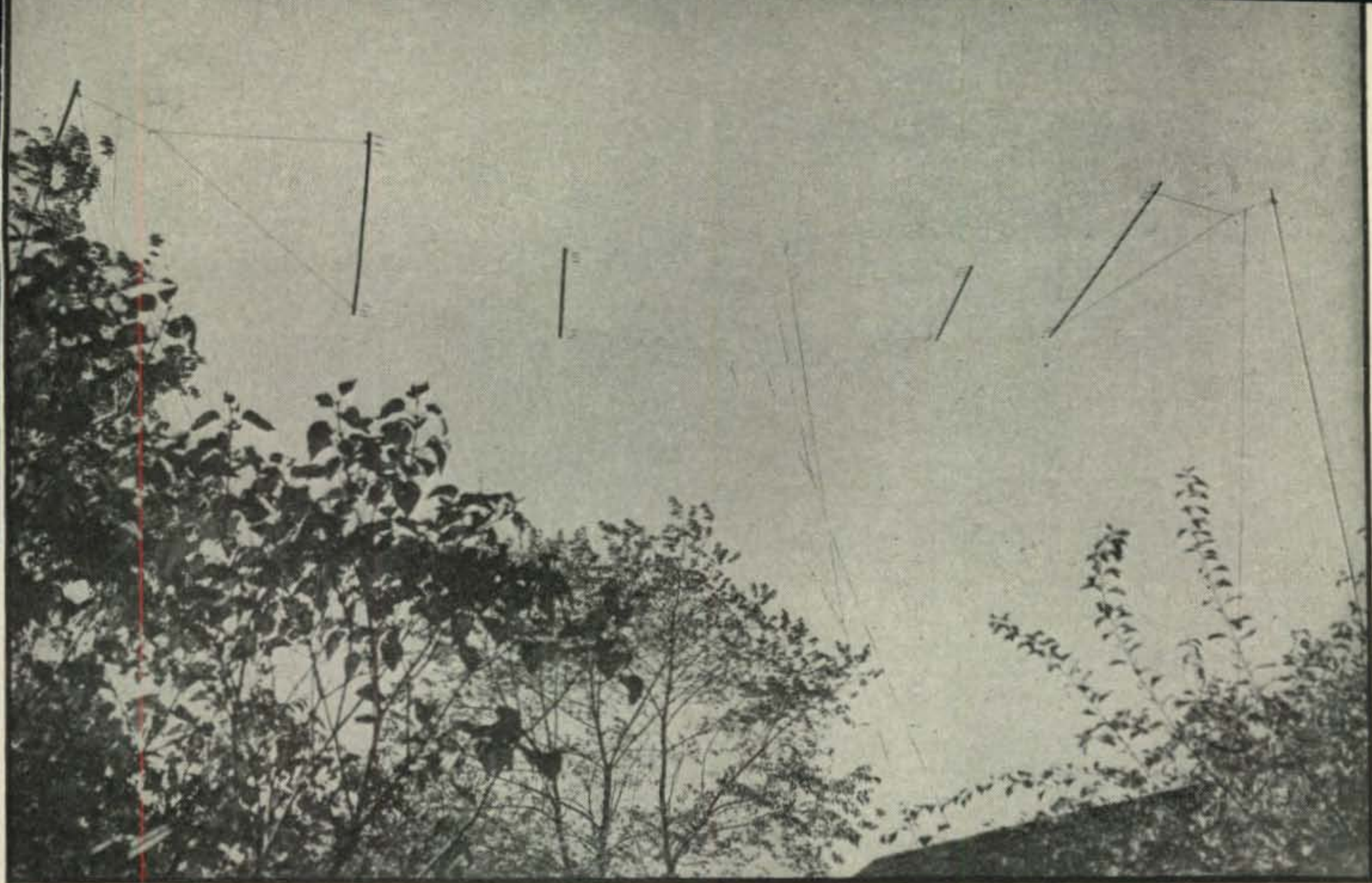
The 20-meter beam with a 10-meter model suspended in the center. No apparent performance change resulted in this space-saving arrangement of the two beams.
