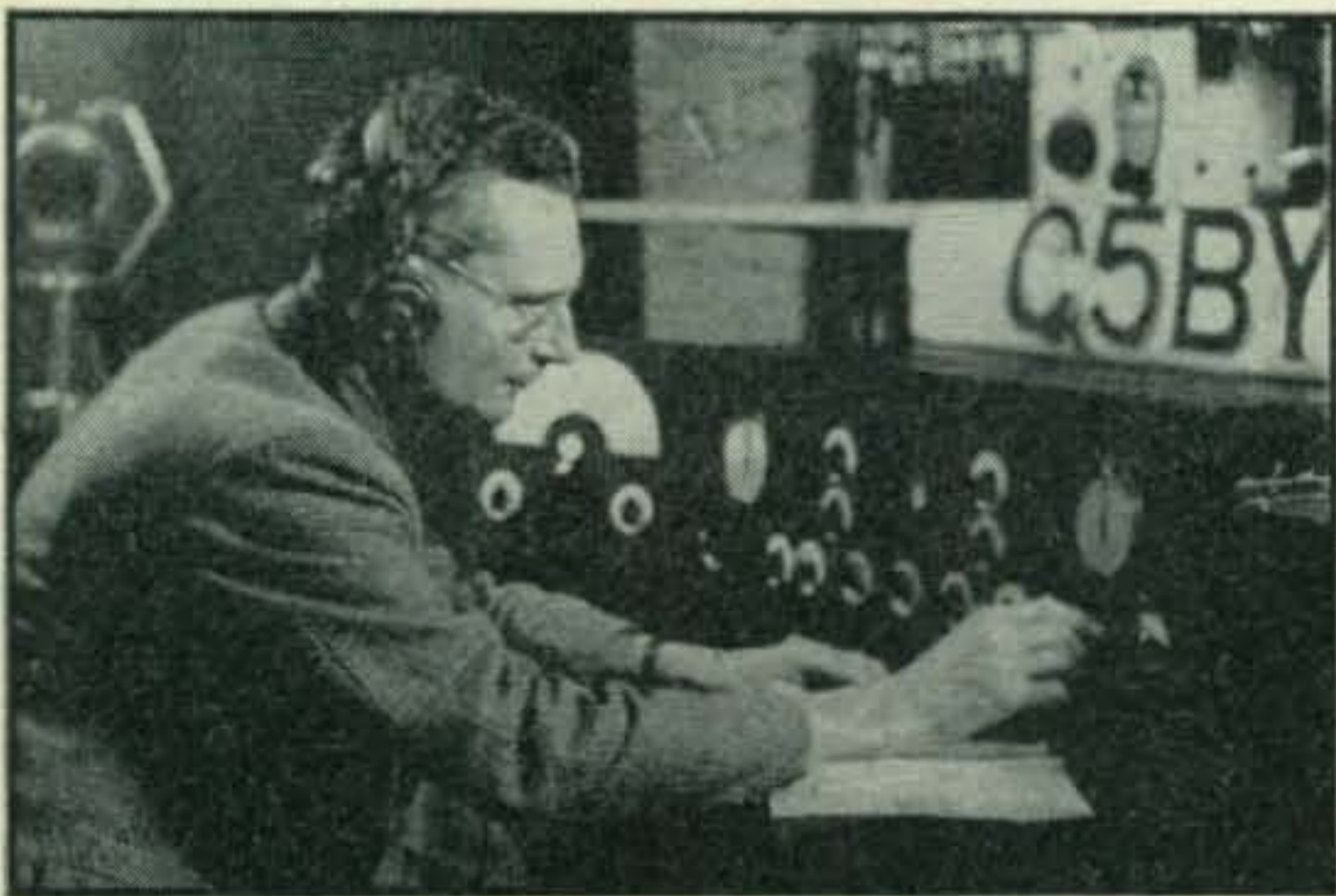
Hilton, G5BY, at his receiving position. Converters, left to right, cover 50-54 mc 56-60 mc, 28-1.7 mc. (plug in coils). G5BY was the first station to log W1HDQ on 50 mc.
