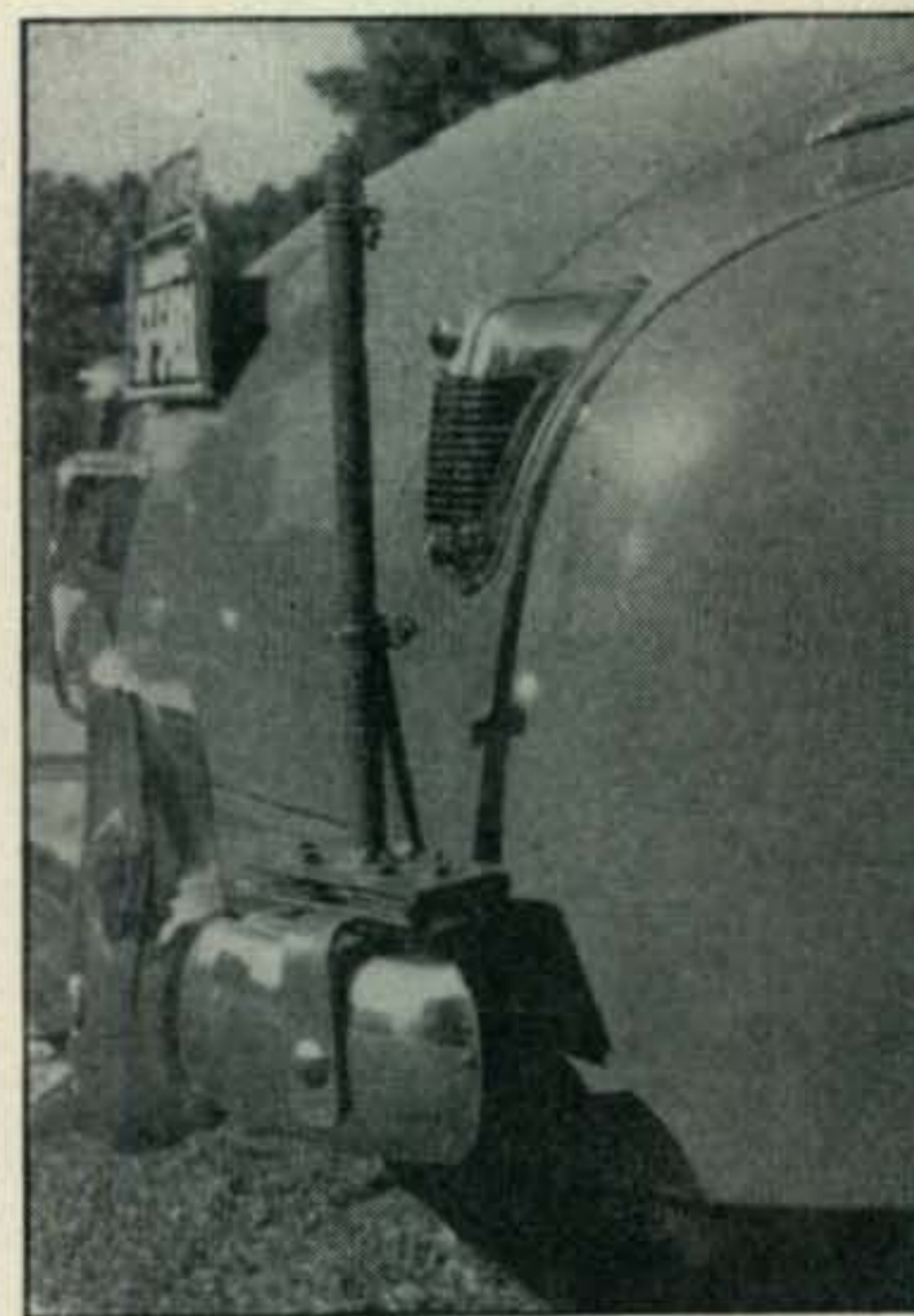
Fig. 2. Closeup view of the insulated antenna base for the tank type antenna.
