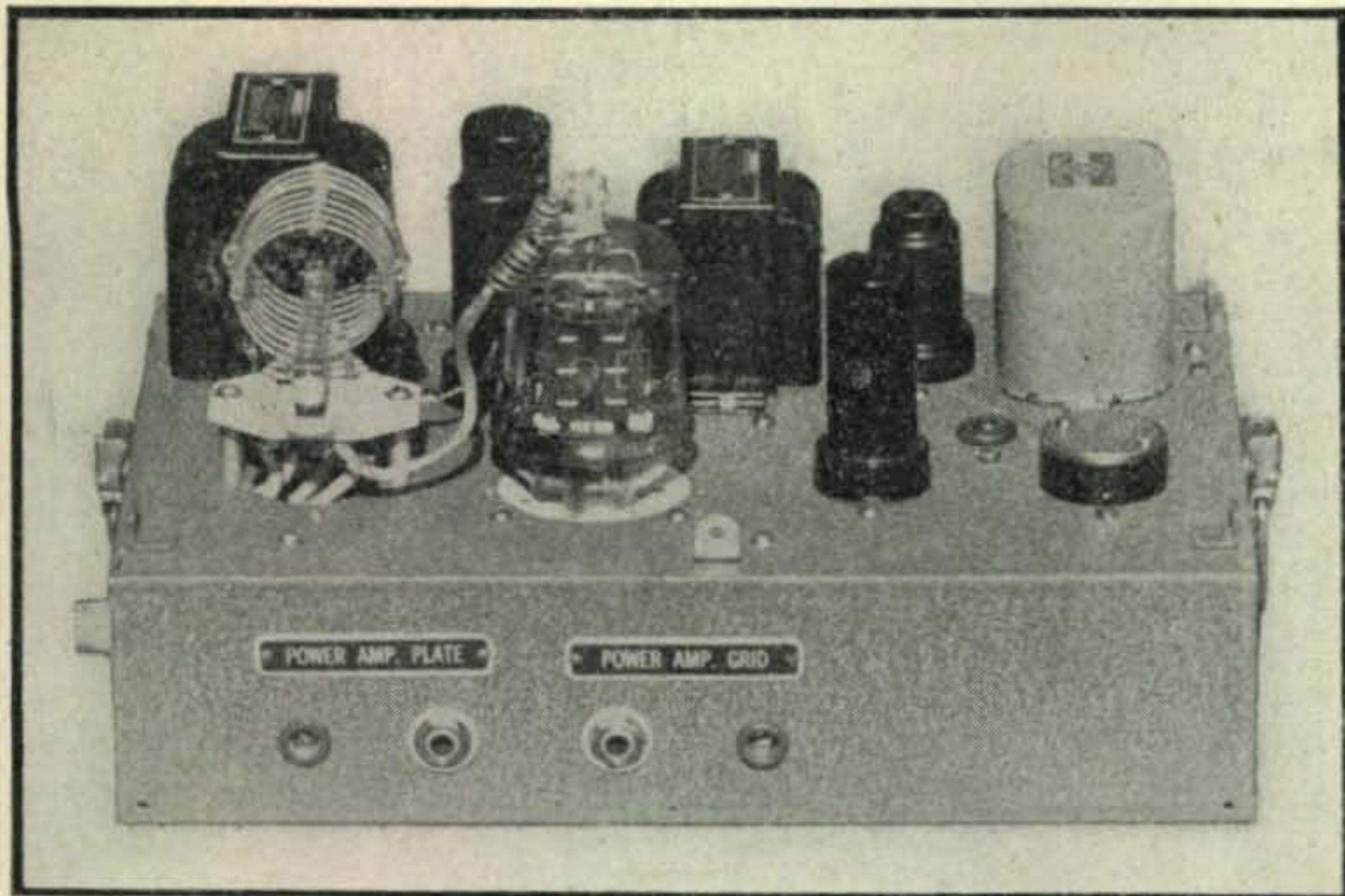
❖ ❖ Fig. 4. Top view of the mobile transmitter. The name plates cost little but add much to the beauty and workmanship of the finished article. ❖ ❖
