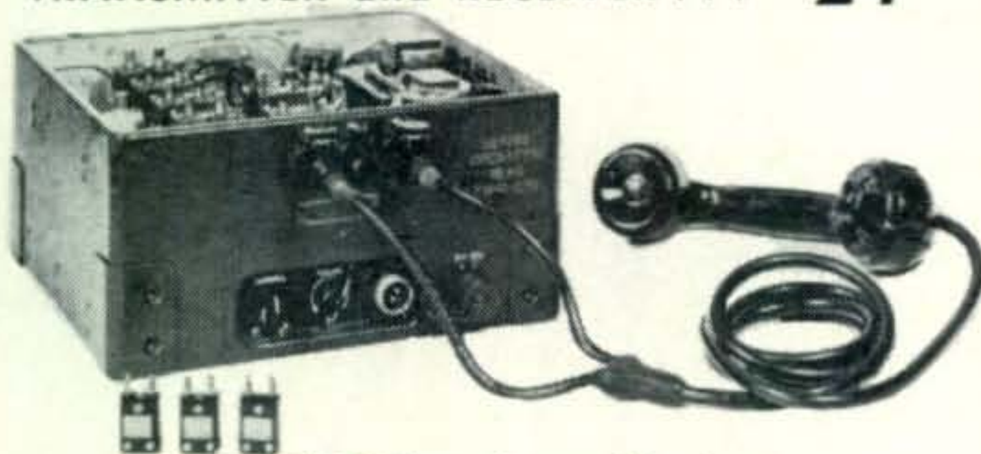
BC 1335 FM Transmitter and Receiver (Choice of one xtal free with each unit)
