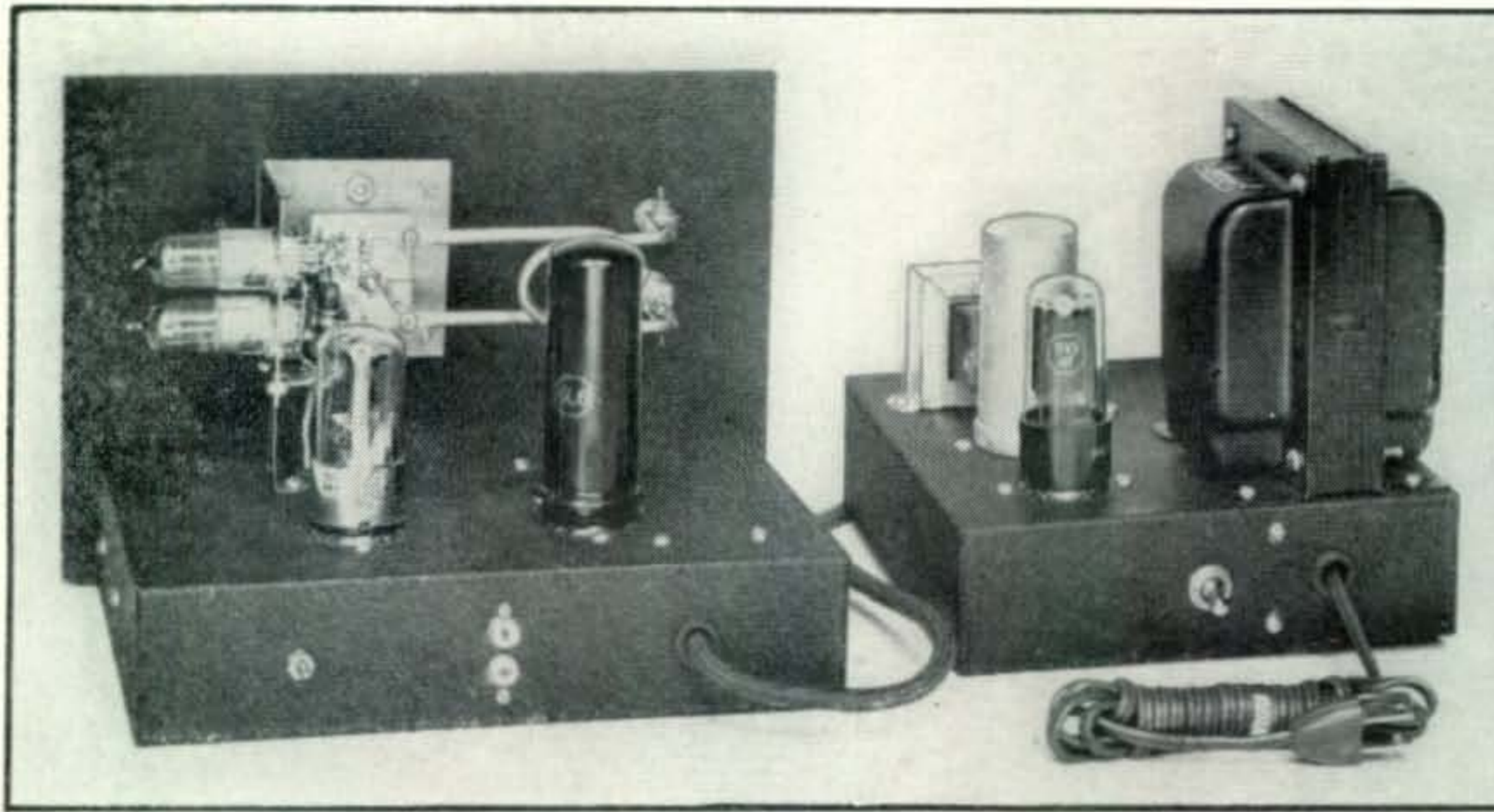
Photograph D. Rear view of the v-h-f transmitter and its associated power supply. Left to right along the rear apron are: The ground terminal, the ceramic tip jacks (a 1/2-inch crystal socket) the power cable and, on the power supply, the a-c On-Off switch and the line cord.
