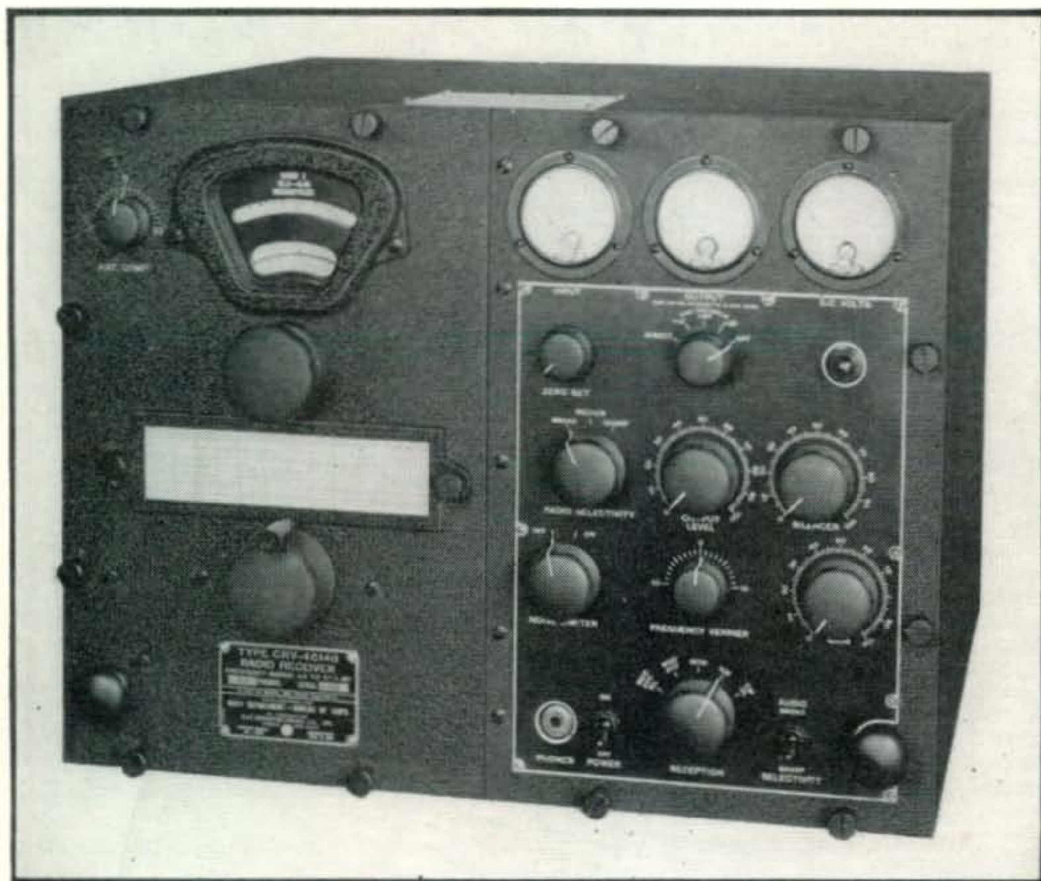
❖ ❖ Navy model RBC high-frequency receiver. The input meter is calibrated in decibels up to 120 above one micro-volt signal input. The center meter is an audio-frequency output meter. The right hand meter reads d-c volts. ❖ ❖
